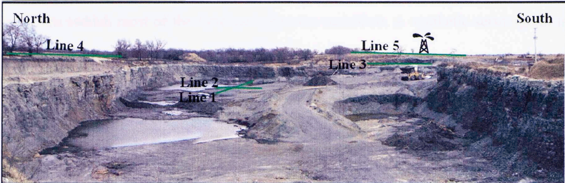
Figure 22. Panoramic view of the quarry, showing the location of the 2D Seismic Lines.
