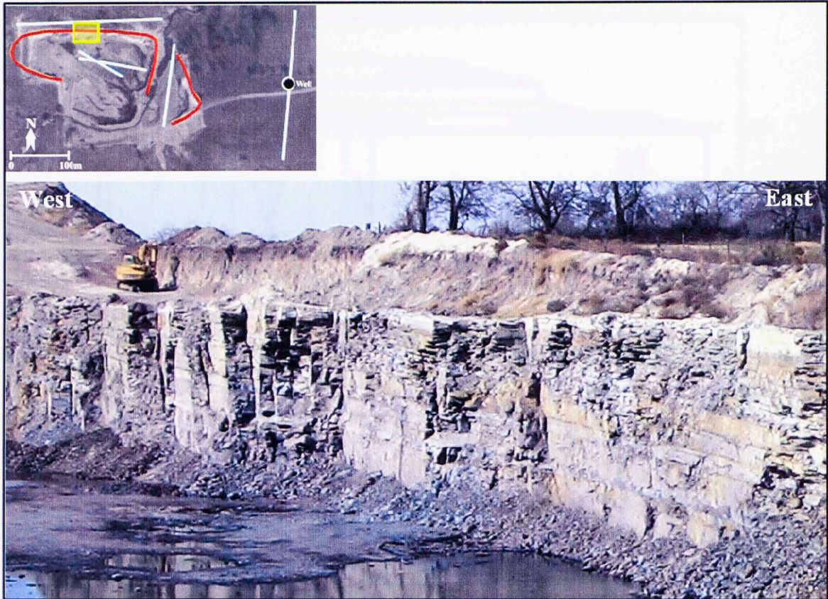
Figure 11. Photo from the Wyche Shale Pit Wall #4 showing fracture planes with approximately west-east strike, possibly representing extensional fractures.
