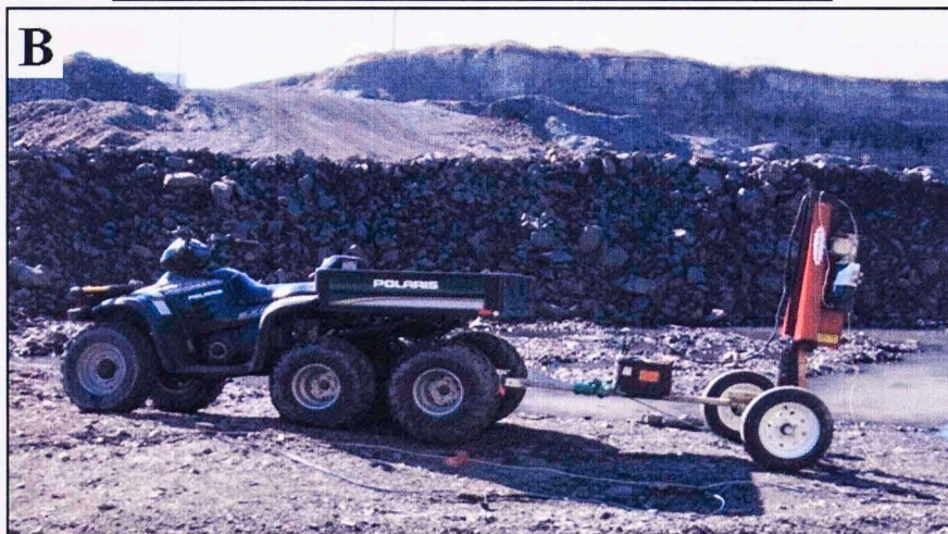
Figure 23. (A) 48-channel Bison Series 9000 Digital Instantaneous Floating Point Signal Stacking Seismograph, and (B) Source, automatic sledge hammer striking an aluminum plate.
