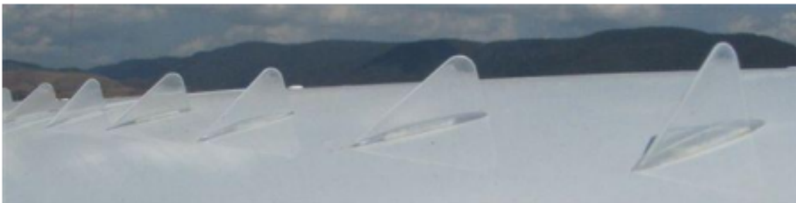
Figure 1: An example of a triangle-shaped vortex generator [3].
