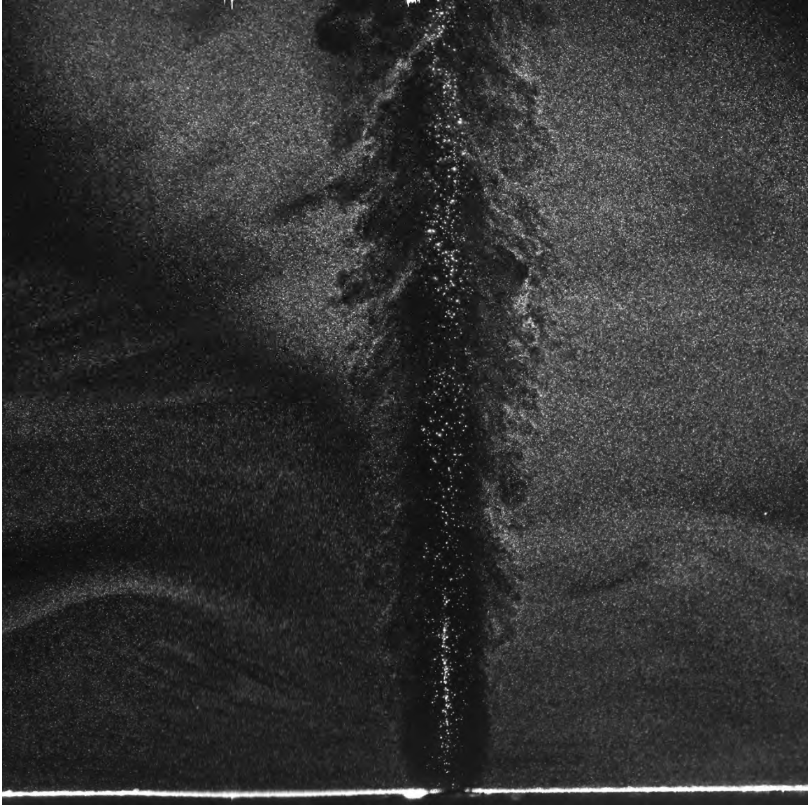
Figure 3.2a.6 - Example of image collected for a vertical ( 0^\circ ) single choked jet nozzle discharging 1[\mu\text{m}] aluminum oxide particles into a water vapor saturated environment.
