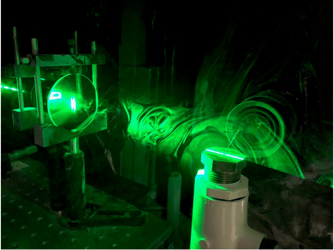
Figure 3.2b.8 – Laser pulse passing through 30° nozzle injection stream perpendicular to the camera lens
