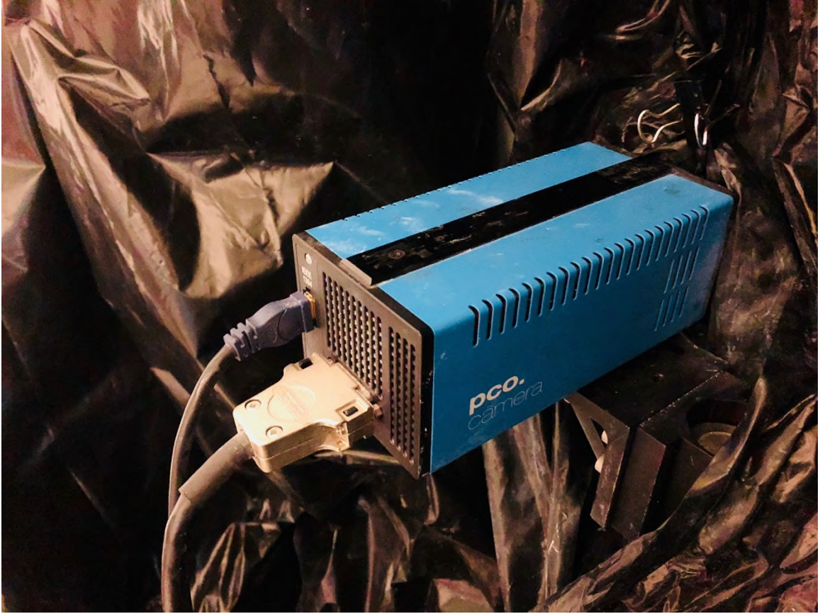
Figure 3.2c.1 – Camera (Model: PCO.2000, Cooled 14bit, 2048 x 2048 pixels).
