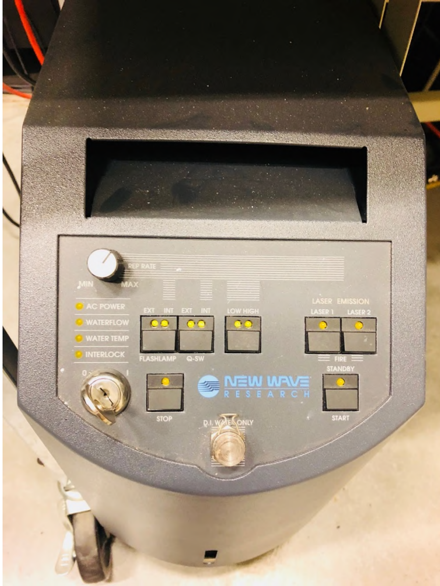
Figure 3.2b.1 – Laser Control Tower (New Wave model: SOLO III PIV).
