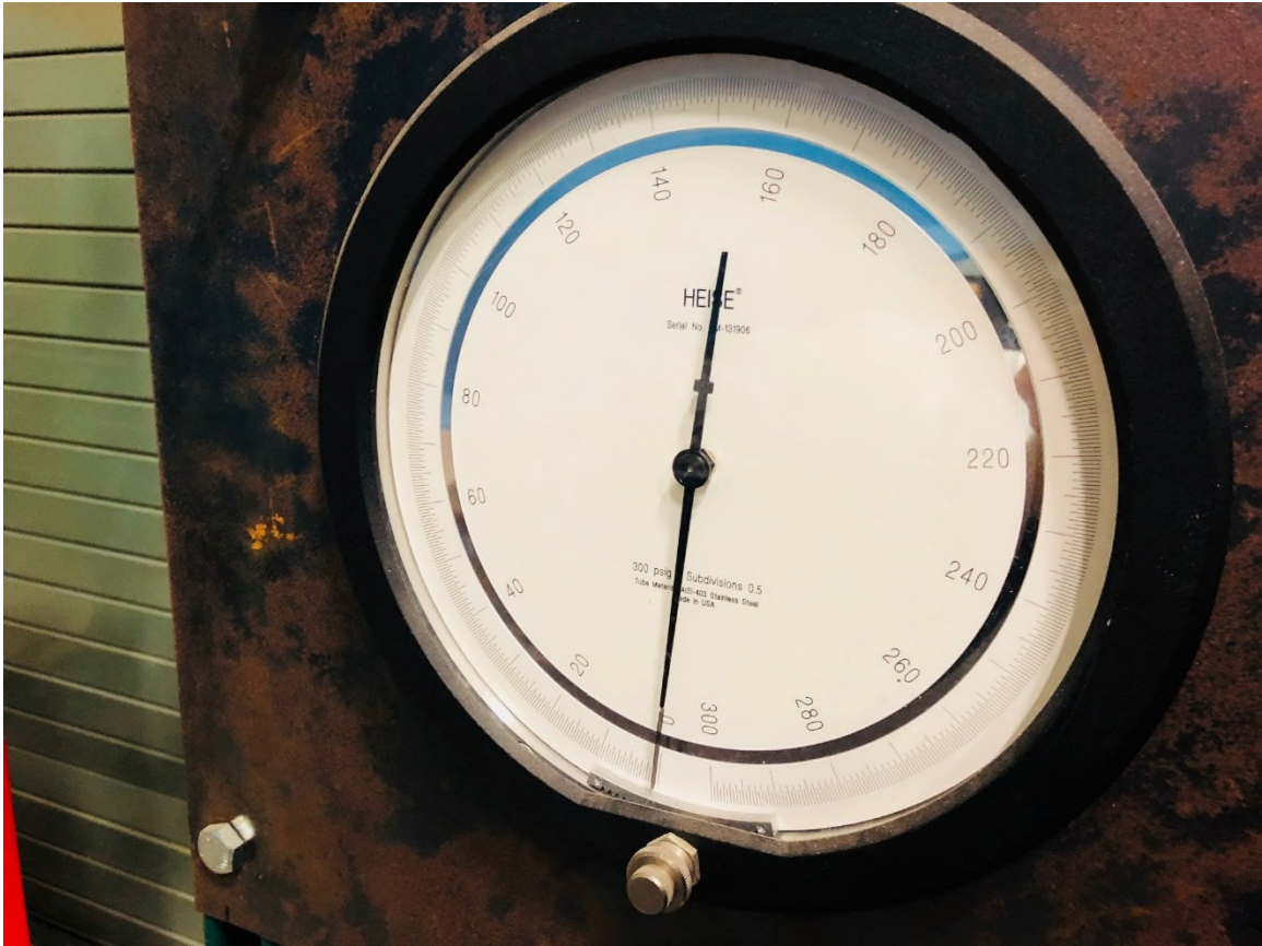
Figure 3.2a.3 – PG-201 pressure gauge measuring the pressure up steam of the nozzle exit.
