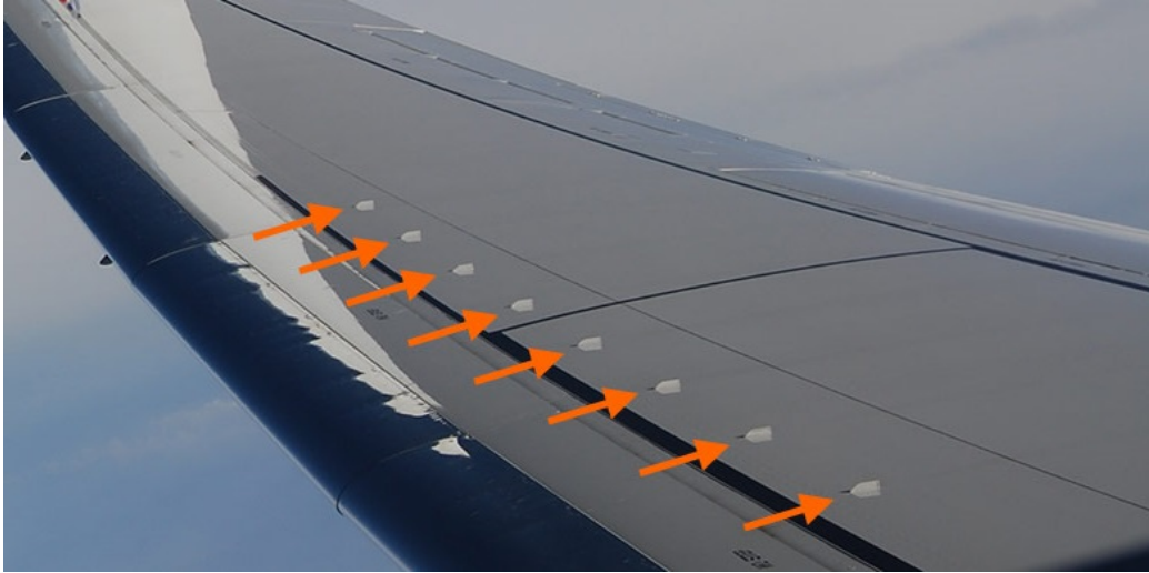
Figure 1: An example of a vortex generators used on a Boeing 737-800 wing [11]
