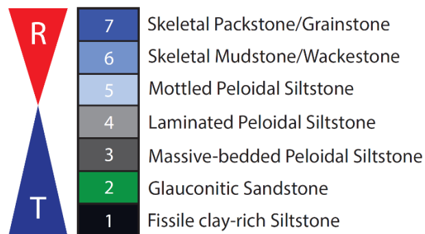
Figure 15: Idealized facies stacking pattern: This study identified 7 primary depositional facies utilizing core and thin section analyses. These facies were placed in a shoaling upwards progression. The blue triangle represent the transgressive portion and the red triangle represent the regressive portion of one rise and fall of relative sea level.
