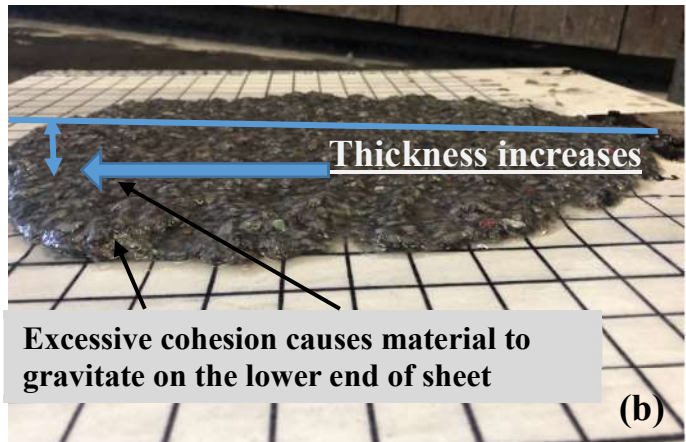
Figure2-17: (a) Table showing the uniform coverage of Pulp Cure with a Spread of 13 inches. This indicates the flow is increasing. (b) The picture shows the thickness increasing towards the lower end of the slope.
