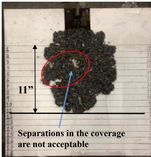
Figure2-14: The figure shows separations in the Spread, revealing the white sheet beneath. This would not be acceptable performance. Addition of tackifier would solve this issue.
