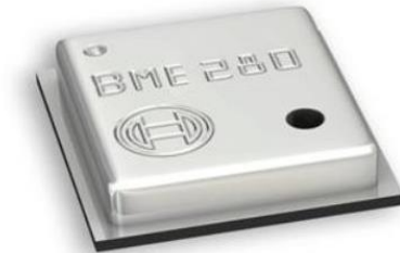
Figure 29: BME 280 Environmental Sensor
