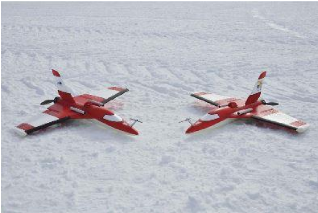
Figure 13: Small Unmanned Meteorological Observer (SUMO) unmanned aerial vehicles (UAVs) at Williams Field Antarctica [23]
