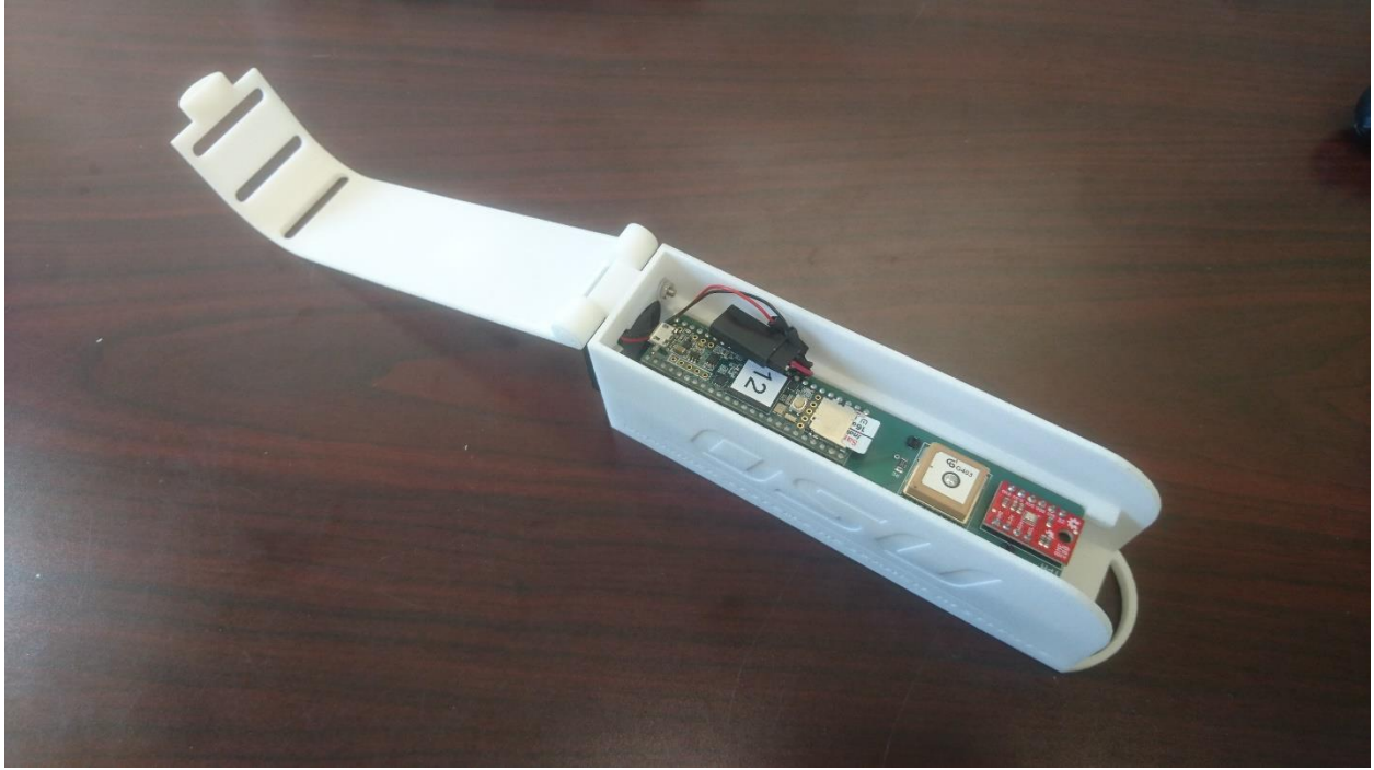
Figure 34: Dropsonde housing open
