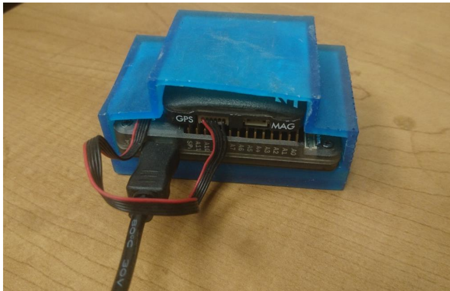
Figure 26: Ardupilot and GPS in housing
