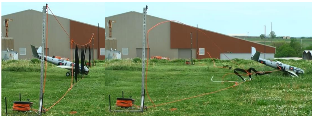
Figure 56 : Pitched Down Recovery Test
