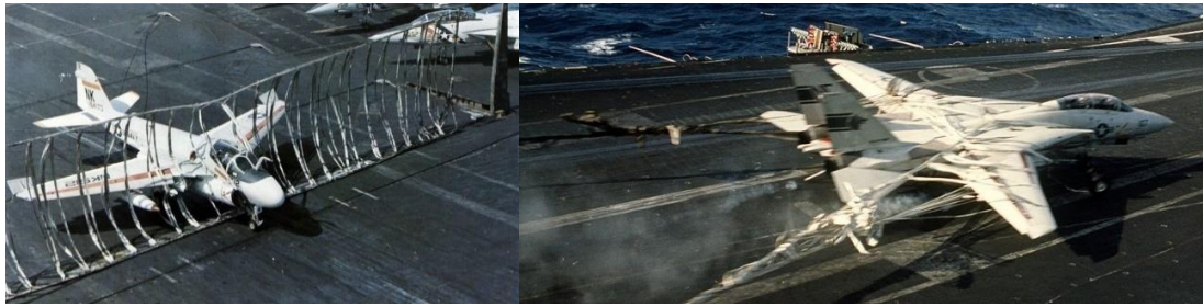
Figure 19 : Carrier Barrier System
