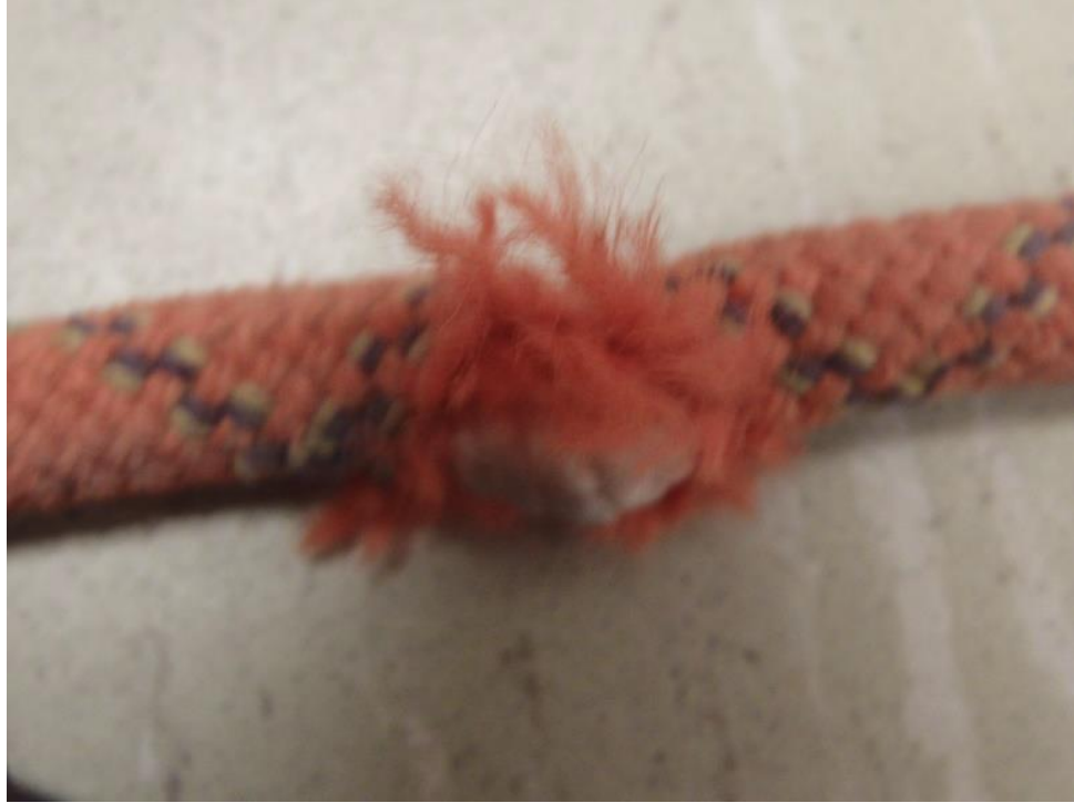
Figure 81 : Close-up of Top Rope Damage
