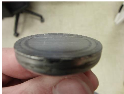
Figure 91 : Magnet with Divots Filled with JB-weld
