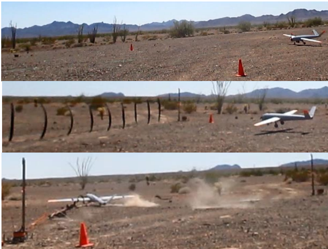
Figure 60 : 7/14/2015 Off-runway Successful Recovery with Minor Damage
