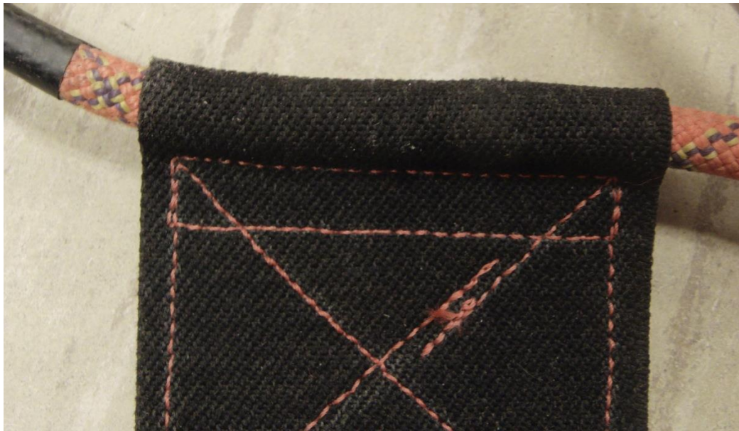
Figure 76 : Example of Strap Ripped Free
