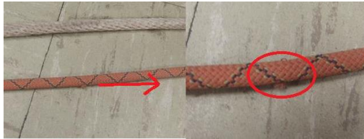
Figure 71 : Addition Example of Stitching Left Over from Modification
