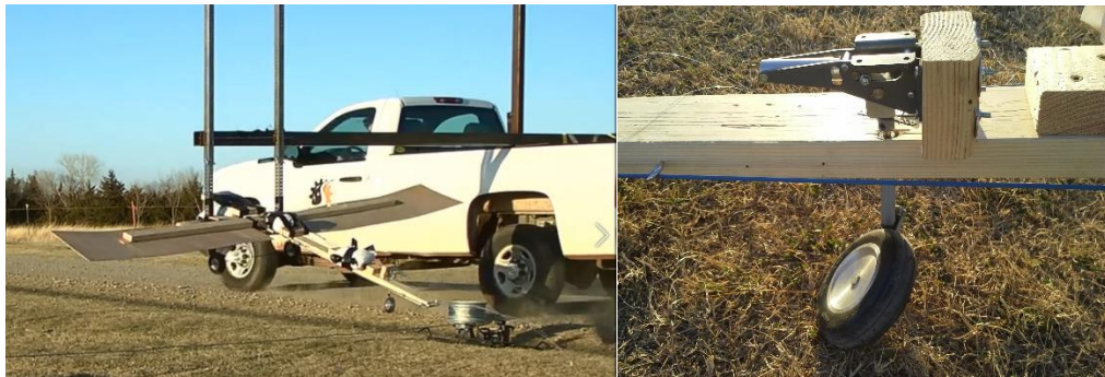
Figure 47 : Analogue Tilting and Gear Damage
