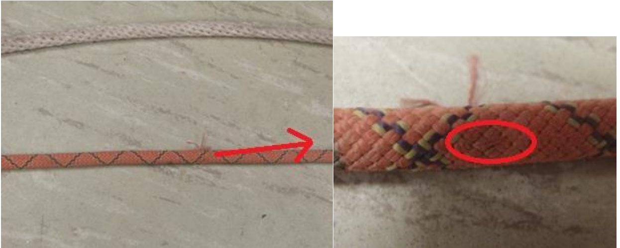
Figure 70 : Threads on Bottom Rope Confirmed as Stitching Left After Modification
