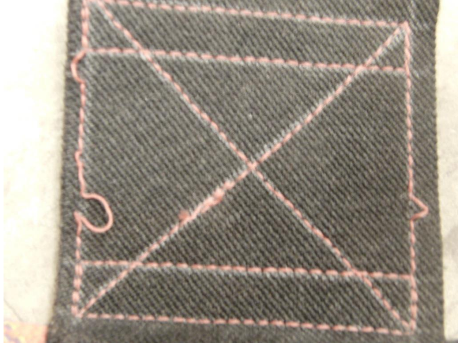
Figure 77 : Strap 4 Loop Stitching Damage
