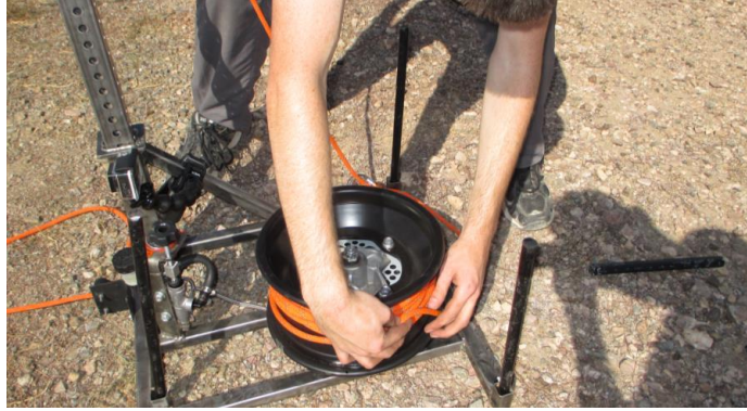
Figure 0-7 Reeling in Dissipater Rope
