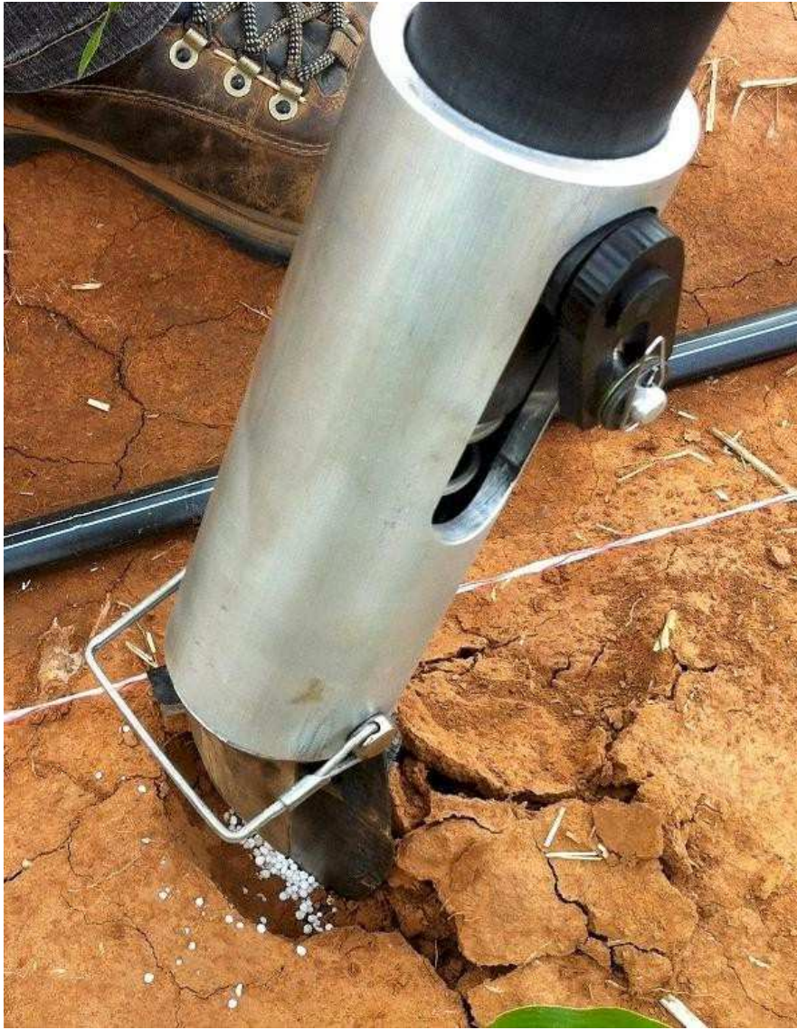
IMAGE 2. A closeup of the hand planter head, to illustrate urea nitrogen application during a strike to the soil. Source:
