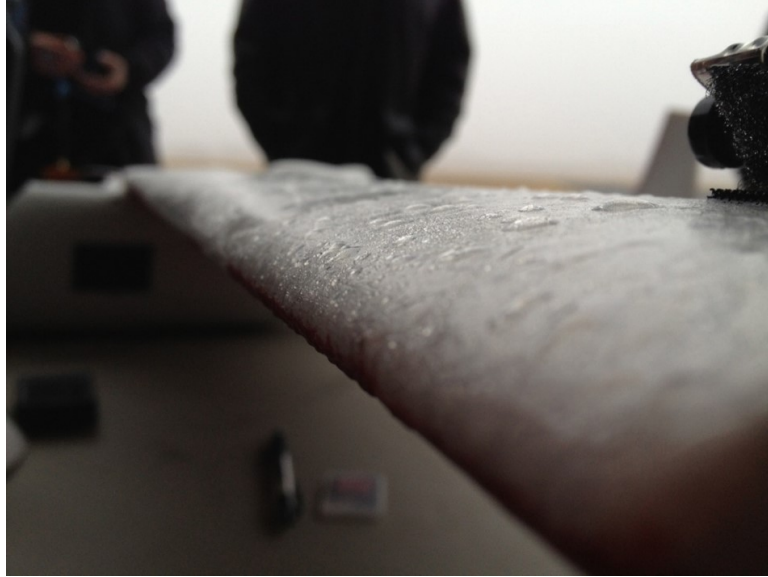
Figure 1.1: Ice accreted on one of Oklahoma State's UAS on a routine test flight.
