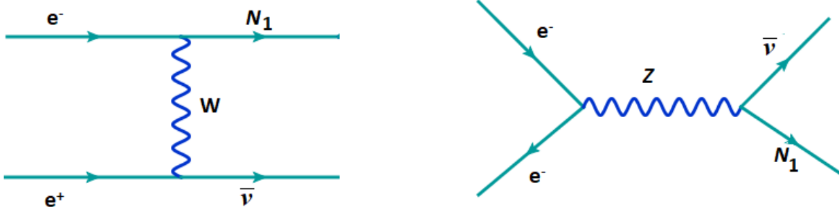
Figure 8.4: RHN production processes at the linear collider. The left panel is the dominant t channel process and the right panel is s channel process to produce the e^+e^- \rightarrow N_1\nu_1 . To produce N_2\nu_2 and N_3\nu_3 , the Z mediated s channel process will act.
