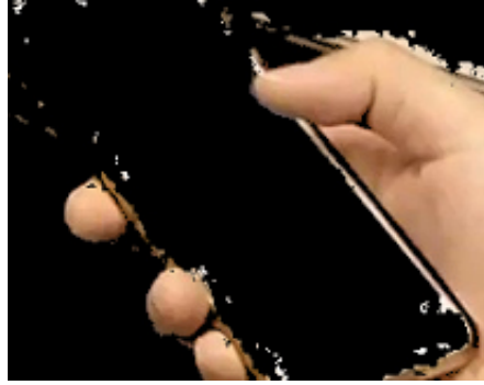
Figure 2.3: Image of the ROI showing the person's hand. The person's skin color is filtered out to obtain the contour of the finger.
