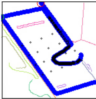
Figure 2.4: Final image where the contour of the smartphone screen, the contour of the finger, and the number keypad can be clearly seen.
