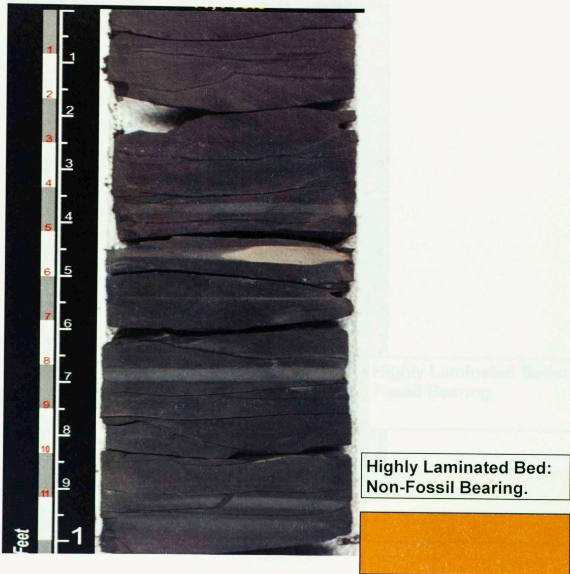
Figure 3.8: Highly laminated Beds: Non-Fossil bearing example. Grey and white scale: inches. Photos provided by Core_Lab, Inc.
