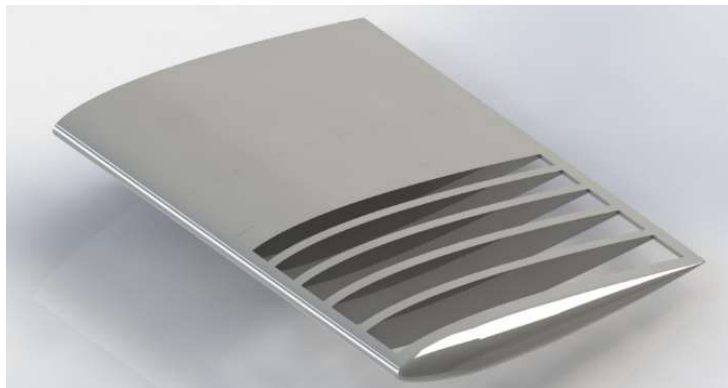
Figure 3: Modified NACA 0012 airfoil with slits
