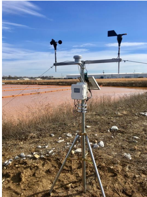
Figure 2.3 HOBO U30 USB Weather Station deployed near northwestern corner of oxidation pond to collect wind data
