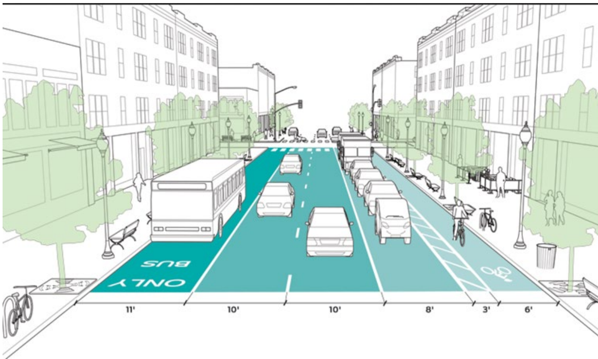
Figure 2.2 Lane Width Guide (NACTO 2017) where image shows only initial building development not potential building height
