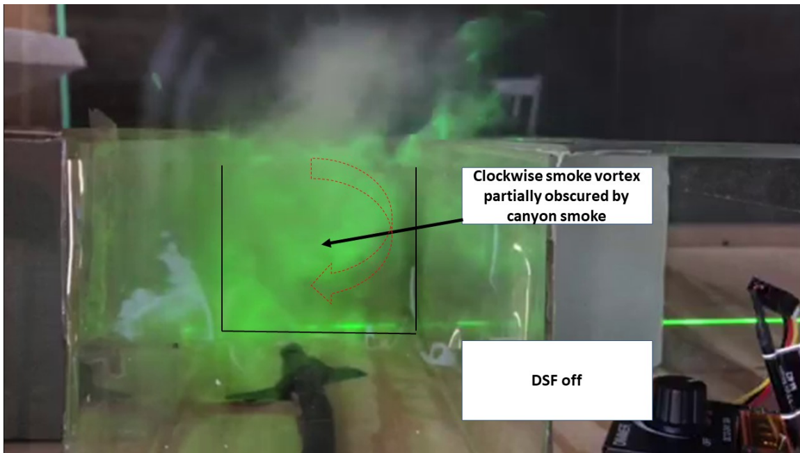
Figure 5.5.5 Cold Smoke 0:09s Smoke Entering Recirculation Vortex Apparent
