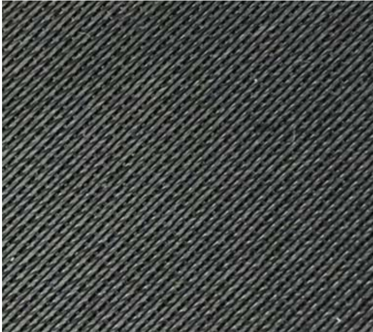
FIGURE 4. 7 Bottom of Fortus 450 test block showing surface quality.
