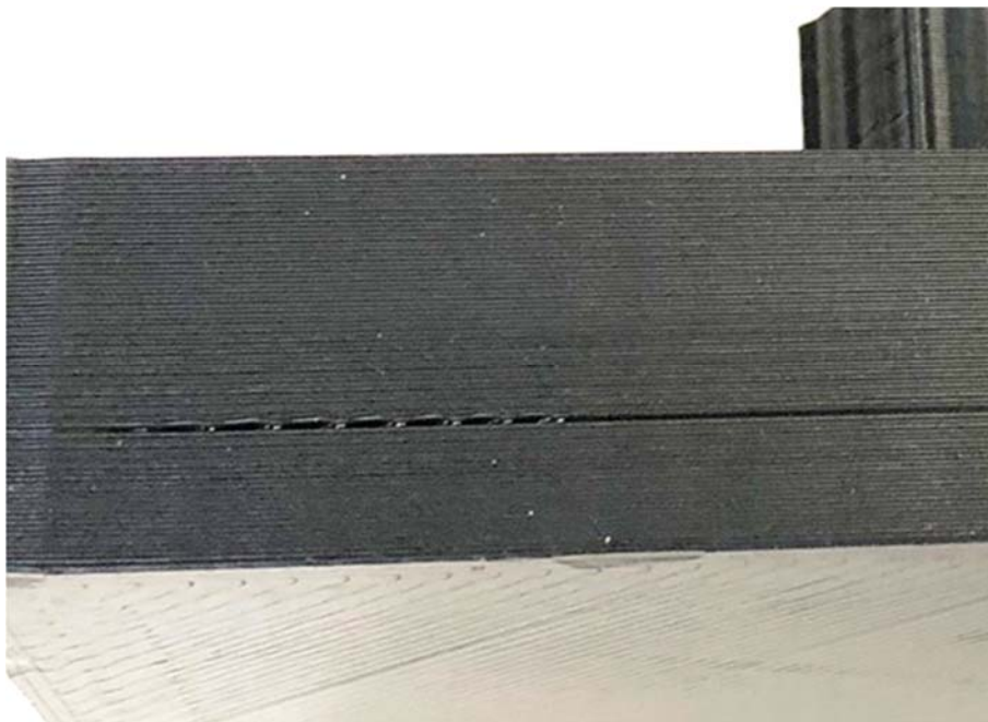
FIGURE 4. 3 Gap in filament layer on front side of 3D Platform block 1
