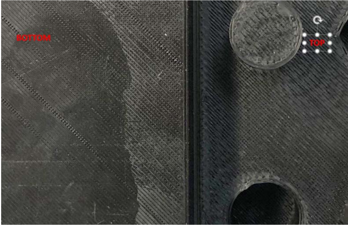
FIGURE 4. 6 Bottom and Top f 3D Platform test block showing surface quality.
