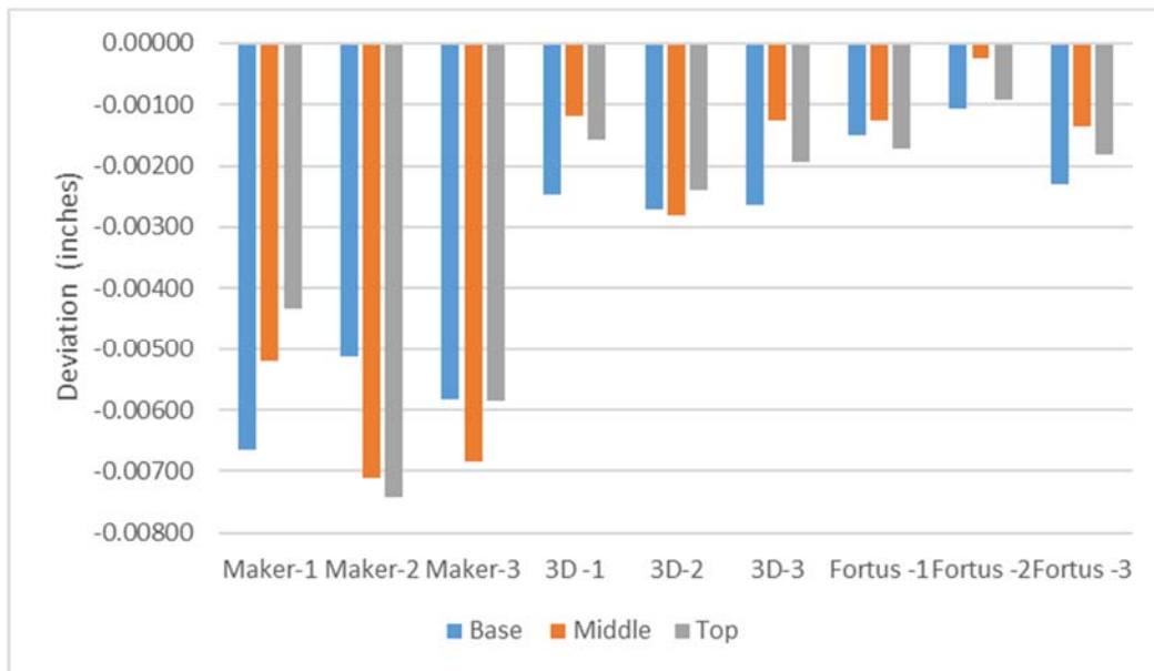
FIGURE 4. 10 Raised cylinder diameter deviation from CAD model diameter of 0.75 inches
