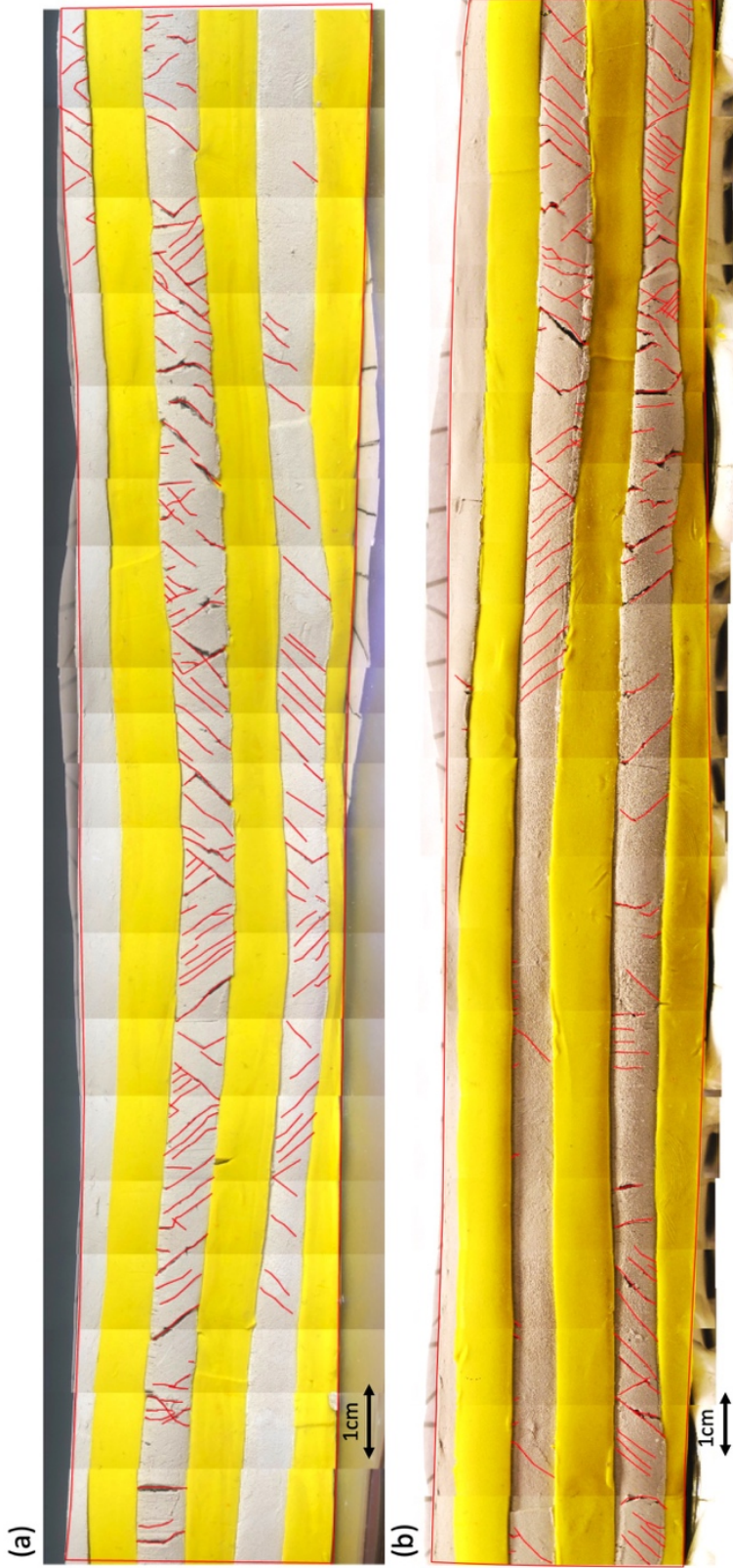
Figure 4.9: Layer clay model with 1cm thickness, the measured areas are outlined by red lines and the fractures are delineated by red thin lines.
