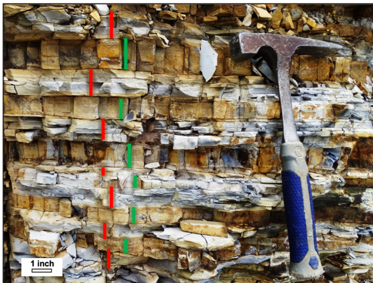
Figure 3.2: Interbedded chert and siliceous organic-clay shale on the I-35 outcrop. Red lines outline the siliceous and clay/organic rich shale that is weathered to light gray on the outcrop; green lines outline the chert beds that are massive and brittle. Note that most of the fractures are bed-bounded in the cherty beds but not extend to the siliceous shale, and density varies on these two different facies (Becerra, 2017).
