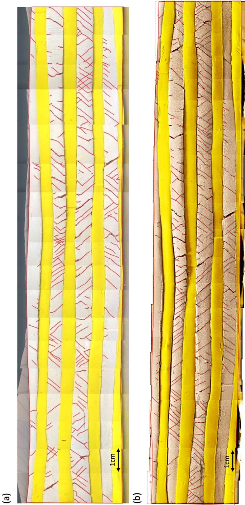
Figure 4.10: Layer clay model with 0.75cm thickness, the measured areas are outlined by red lines and the fractures are delineated by red thin lines.
