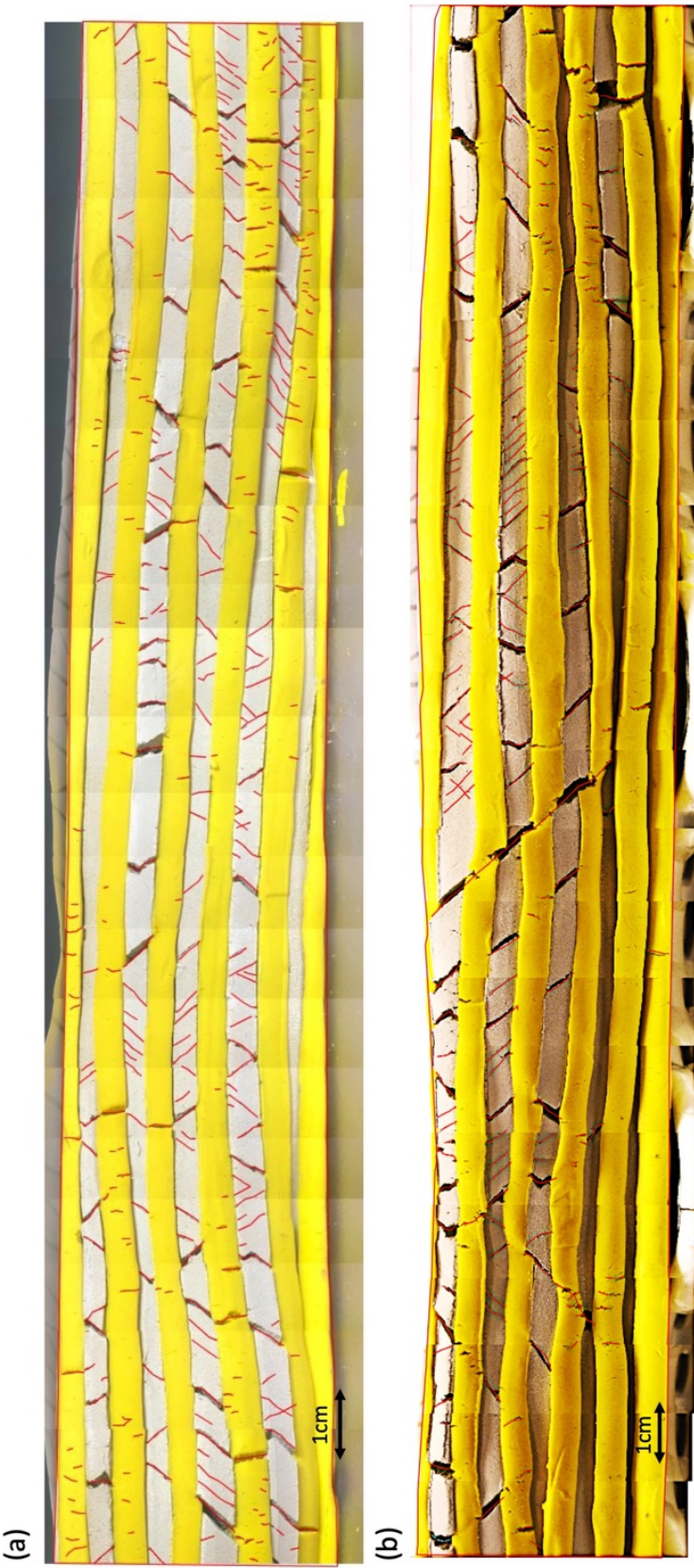
Figure 4.11: Layer clay model with 0.5cm thickness, the measured areas are outlined by red lines and the fractures are delineated by red thin lines.
