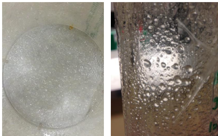
Figure A.20 Oil and water deposition on inner surfaces, counted in losses
