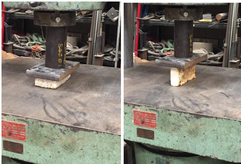
Figure 56: (left to right) Bricks O1 (5% glass) tested horizontally and O2 (10% glass) tested vertically for Compression
