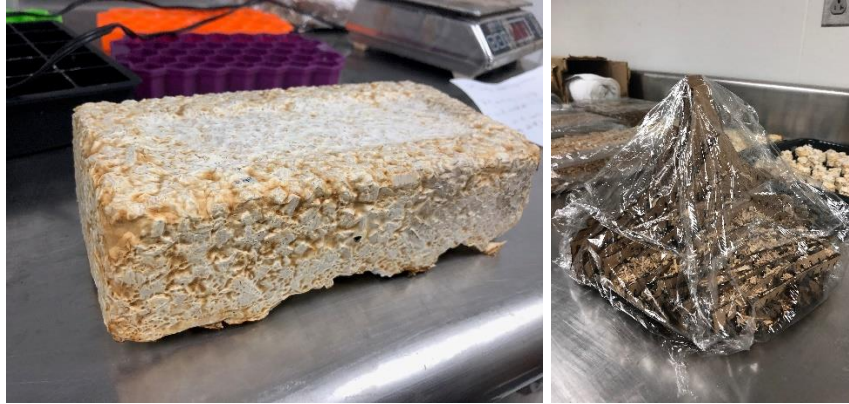
Figure 78: (left to right) A single solid Mycelium brick; Mycelium still growing on cardboard 3D matrix
