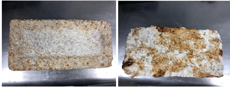
Figure 99: (left to right) Top and bottom surfaces of Mycelium bricks; top surface shows denser material growth, bottom surface shows more porosity because of air pockets
