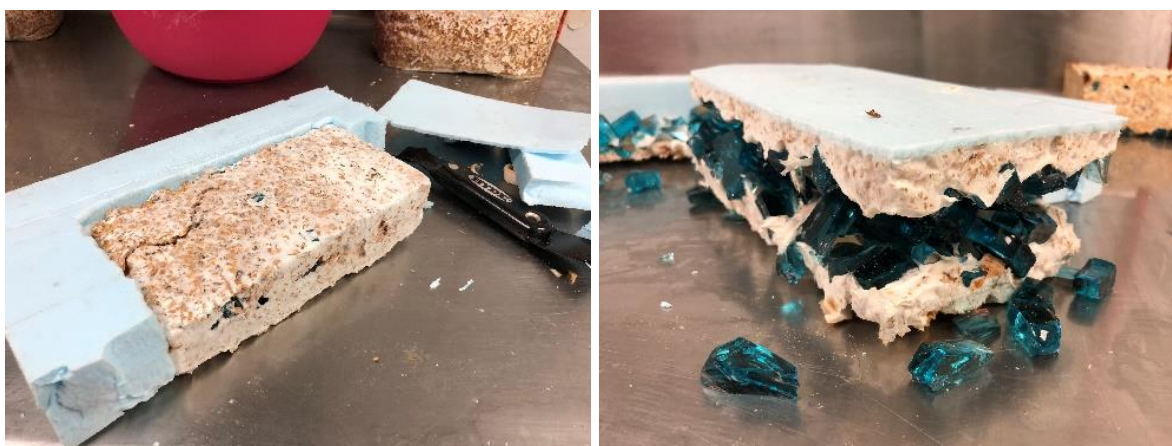
Figure 75: (left to right) Bricks developing cracks; Bricks with higher percentages of glass breaking off from structure
