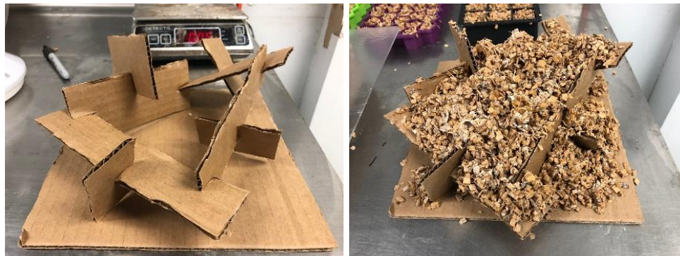
Figure 64: Mycelium material allowed to grow on cardboard matrix for Adhesive Test
