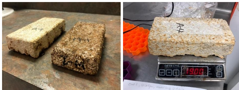
Figure 93: (left to right) Mycelium blocks after being soaked for 24 hours: Brick H1 (Hemp, right) was tested for Absorption test after being mechanically transformed underload by the UTM, and brick A1 (Aspen, left) grown during Test IV; Bricks weighed on digital scale
