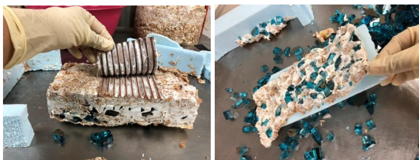
Figure 76: (left to right) Image showing cardboard sheet peeling off from structure without bonding; Composite Mycelium glass brick with 80% glass having a structural breakdown
