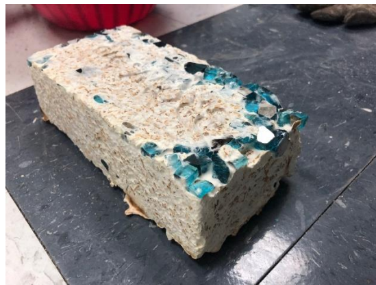
Figure 72: Composite Mycelium-Glass brick after drying and ready to use
