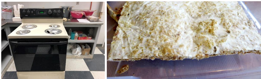
Figure 13: (left to right) Baking oven in Lab; Mycelium block after baking [9]
