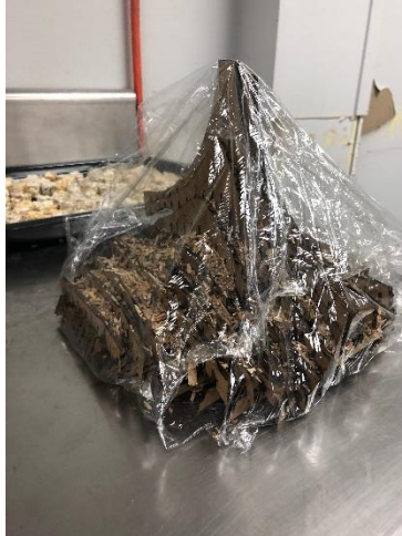
Figure 98: Mycelium material failing to grow on 3-dimensional cardboard structure
