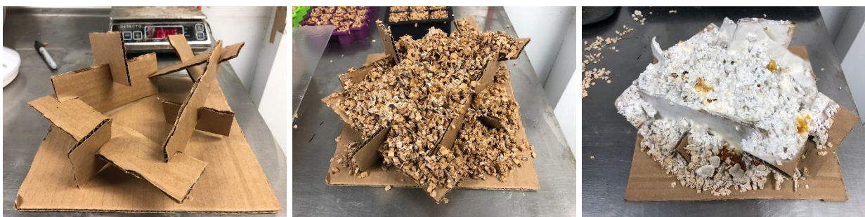
Figure 95: Stages of growth of Mycelium on a cardboard structure demonstrating its adhesive property
