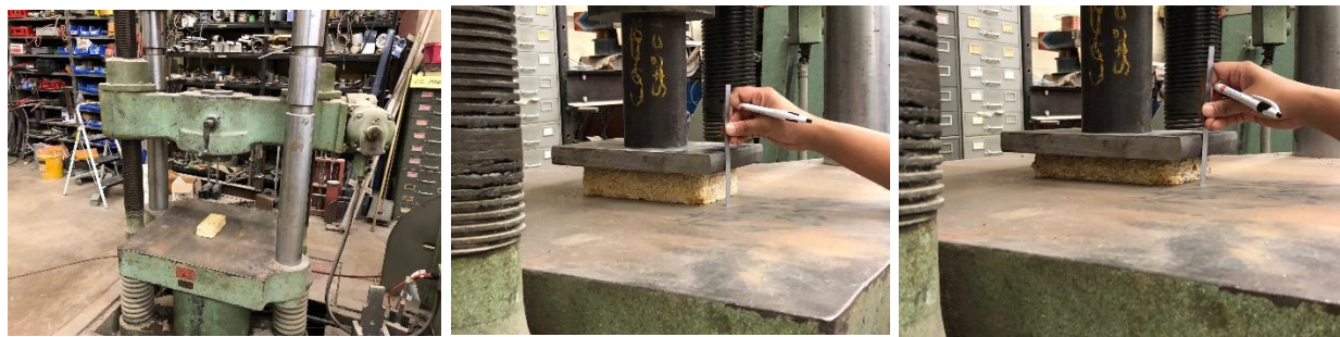
Figure 60: (left to right) Brick H2 (Hemp) tested for Compression horizontally, a gradual shrinkage in depth of the brick is noticed with increase in load without cracking
