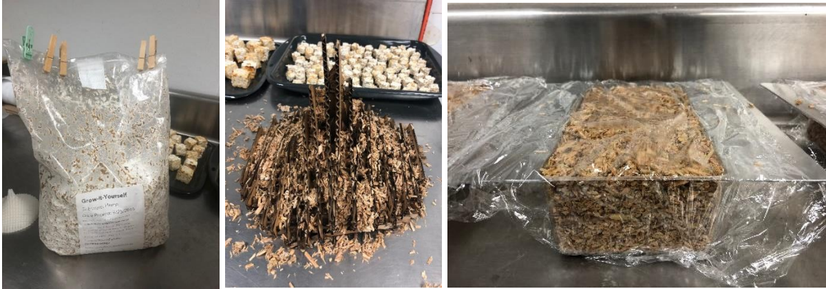
Figure 53 : (left to right) Rehydrated Mycelium(hemp) grows to cover the GIY bag; Mycelium material packed into the 3D cardboard latticed structure; Remaining Mycelium material used to grow more bricks
