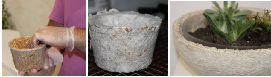
Figure 14: : (left to right) Demonstration of the process of making a Mycelium planter [2]
