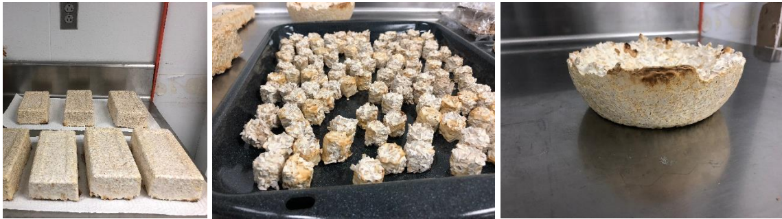
Figure 77: (left to right) Solid Mycelium bricks/ Smaller cubes/ Bowl shaped block of Mycelium formed after Test IV
