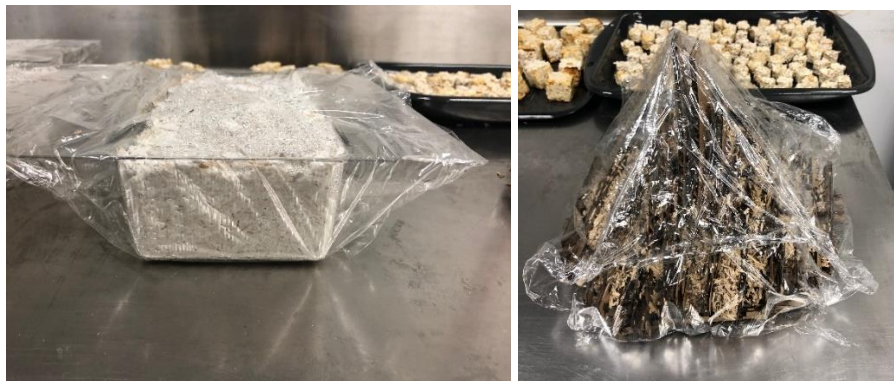
Figure 54 : (left to right) Rehydrated Mycelium growing in brick molds; 3D cardboard latticed structure packed with Mycelium material, still growing and no visible signs of growth of Mycelium/ both observed 4-5 days after start of Stage II
