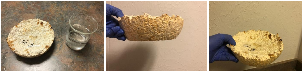
Figure 94: (left to right) Bowl shaped Mycelium block tested for Water Retention Test
