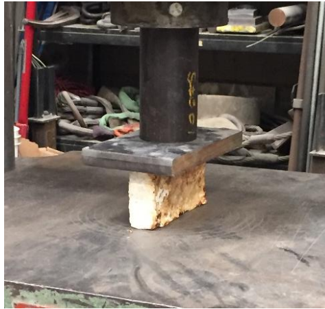
Figure 80: Brick O2 tested for Compression using UTM
