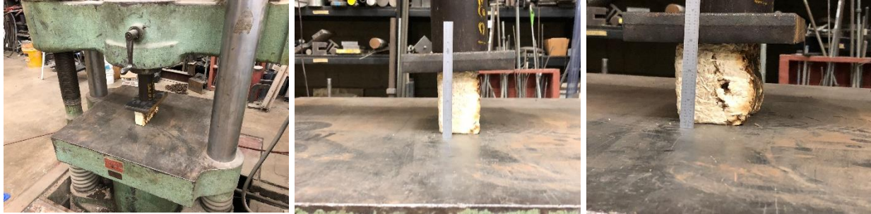
Figure 59: (left to right) Brick A2 (Aspen) tested for Compression vertically, a gradual shrinkage in depth of the brick is noticed with increase in load
