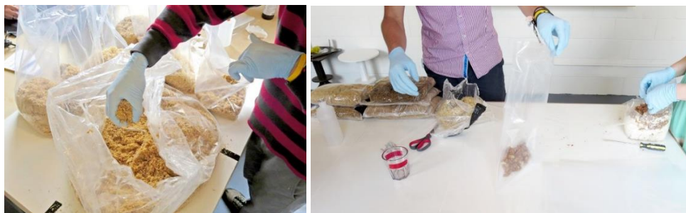
Figure 11: Opening and mixing a bag of Mycelium-based materials/Stage 1 [9]
