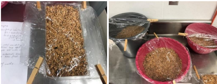
Figure 34: Growth forms packed with Mycelium-based materials at the end of Stage II
