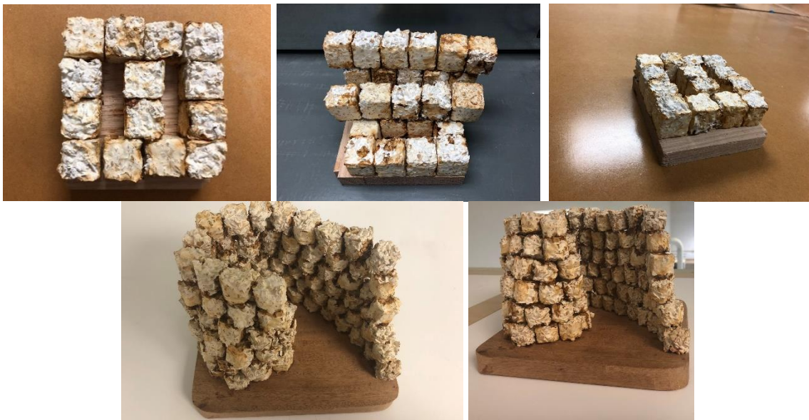
Figure 96: Mycelium block assemblies with straight and curved walls
