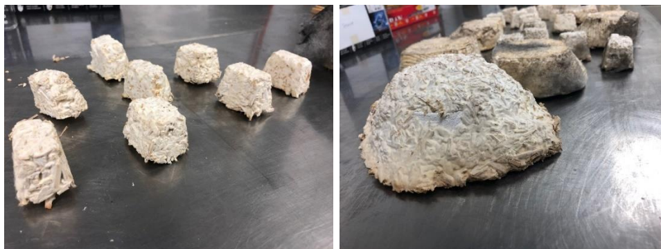
Figure 30: Hemp Mycelium blocks formed at the end of Stage III
