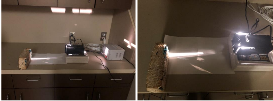
Figure 100: Set-up of Aesthetic Performance Test with Light Box extruding a ray of light which reflects on the surface of Mycelium-glass brick
