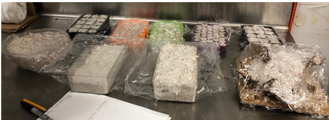
Figure 50: Mycelium material growing in molds, 4-5 days after start of Stage II
