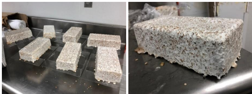
Figure 43: (left to right) Mycelium bricks taken out of molds and ready to be baked; A single brick before drying
