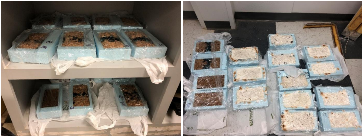
Figure 39: Mycelium material packed with glass in molds; Half of two sets of bricks being inoculated, other half already grown
