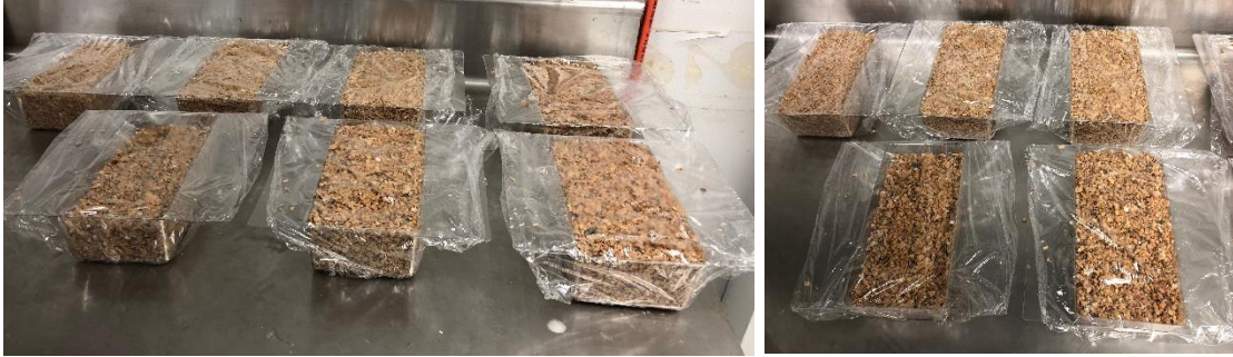
Figure 41: Aspen and Hemp Mycelium material packed in brick molds/ Stage II starts
