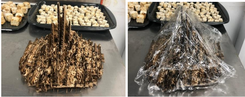
Figure 69: (left to right) Cardboard latticed structure packed with Mycelium material
