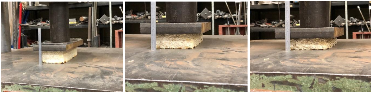
Figure 58: (left to right) Brick A1 (Aspen) tested for Compression horizontally, a gradual shrinkage in depth of the brick is noticed with increase in load
