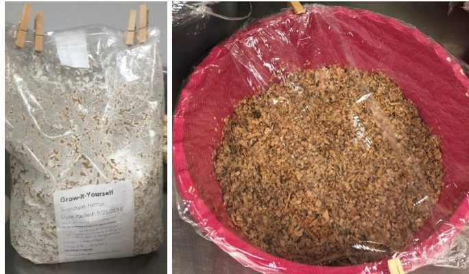
Figure 29: (left to right) Hemp Mycelium showing visible growth turning white; Mycelium packed in plastic bowl growth container at Stage III
