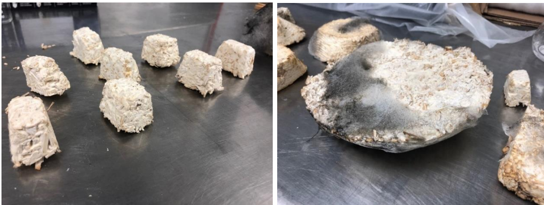
Figure 70: Blocks formed with Plastic molds; a few of them grew molds with time
