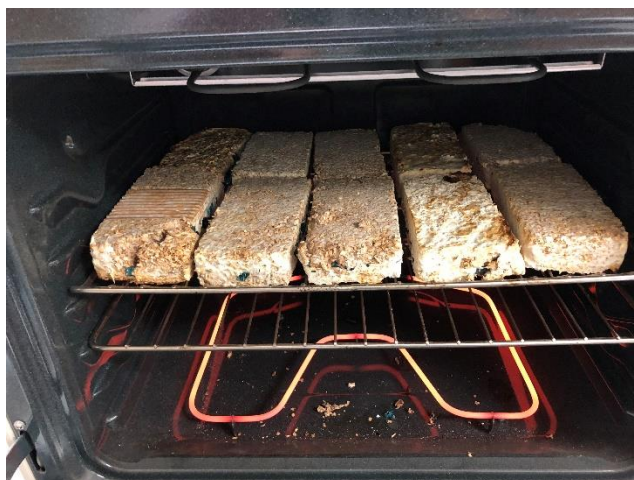
Figure 74: Bricks in oven being baked during Stage III of Test III
