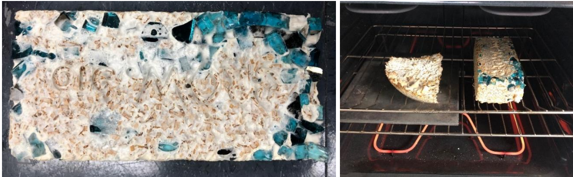
Figure 71: (left to right) A single Composite Mycelium-Glass brick before drying; Blocks being baked in oven
