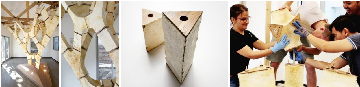
Figure 23: MycoTree, an installation, consists of dozens of mycelium components that support each another in compression. These components are attached to one another with a system of bamboo endplates and metal dowels – but it is the Mycelium that is taking all the load[15]
