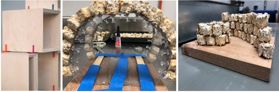
Figure 65 : (left to right) Modular shelf system showing joinery with 3D printed plus connections[18]; Mock-up Assembly Structures made in lab with Mycelium
