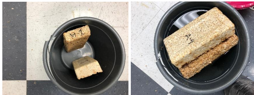
Figure 62: (left to right) Bricks made ready for 24 hour Absorption Test; Testing pail filled with water to perform the Absorption Test
