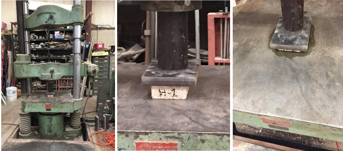
Figure 57: (left to right) Brick H1 (Hemp) tested horizontally for Compression; at a certain load value the brick releases water indicating insufficient drying of brick.
