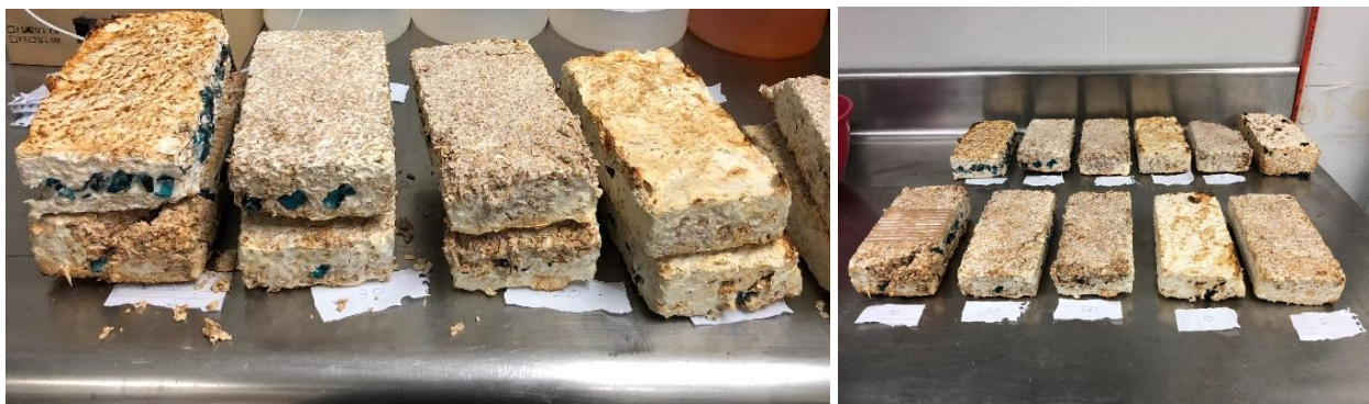
Figure 73: (left to right) Bricks with different percentages of glass formed at the end of Test III
