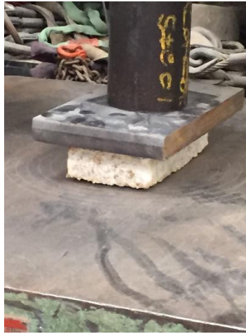
Figure 79: Brick O1 tested for Compression using UTM
