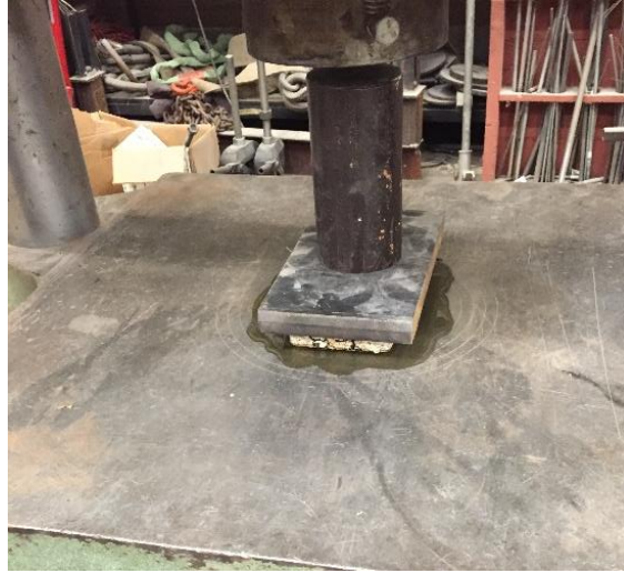
Figure 81: Brick H1 tested for Compression using UTM, releases water under pressure
