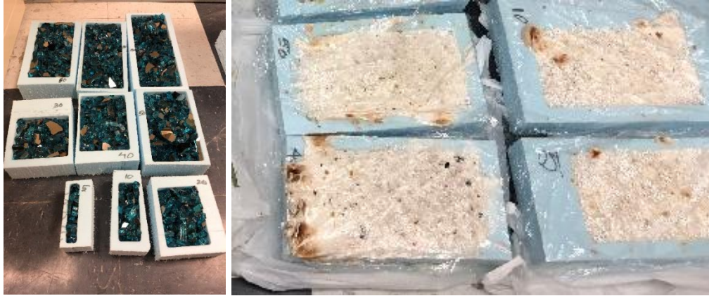
Figure 38: (left to right) Glass filled measuring cups cut out of foam; Mycelium material at the end of Stage 2 after being inoculated, turns white ensuring complete growth of Mycelium.
