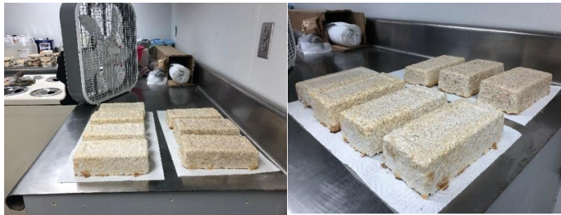
Figure 45: (left to right) Bricks after baking being dried in open by external fan
