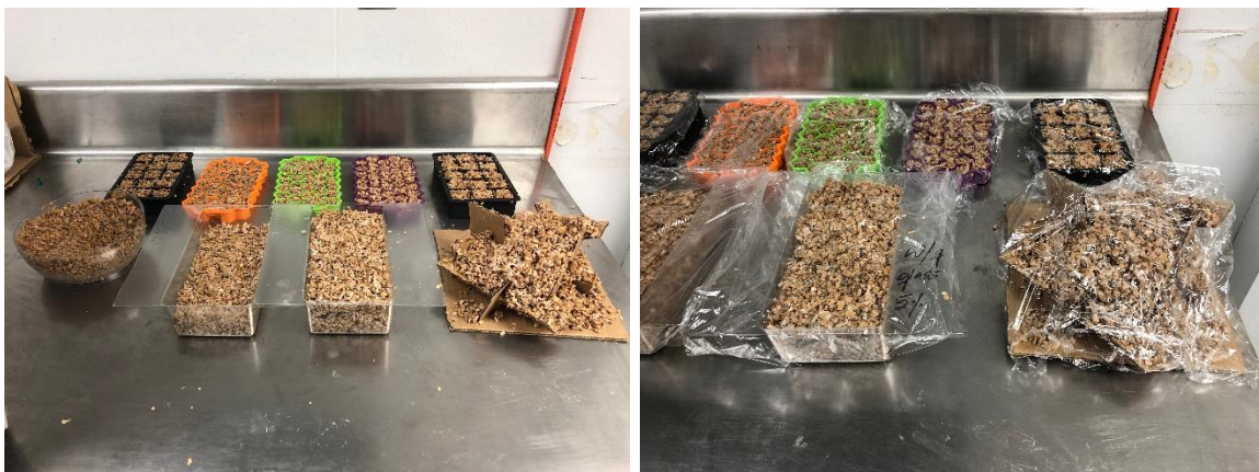
Figure 49: Aspen Mycelium material packed in molds/ Stage III starts
