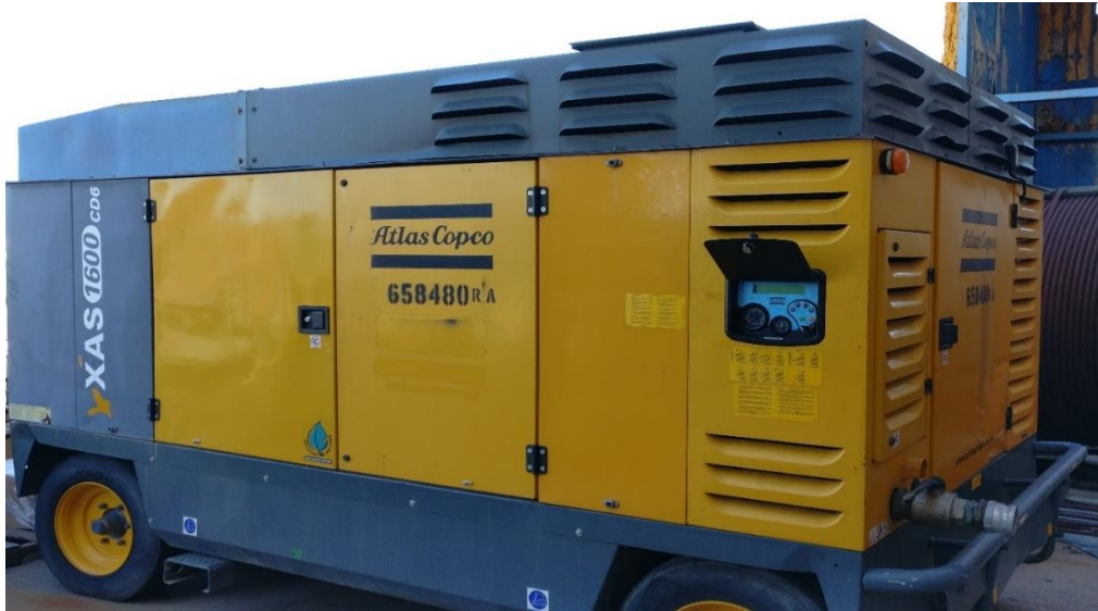
Figure 3.5: Picture of the applied screw-type compressor
