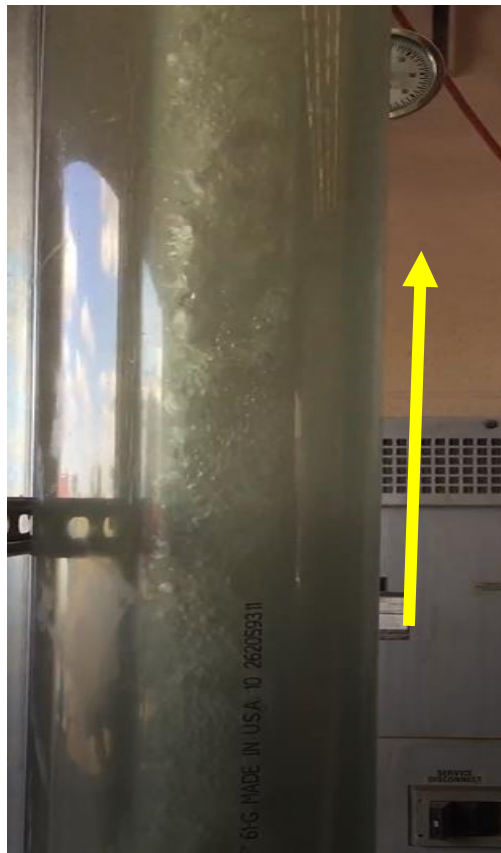
Figure 4.1: Image of fluid flow at 16gpm liquid rate and gas rate of 212,000 scf/day
