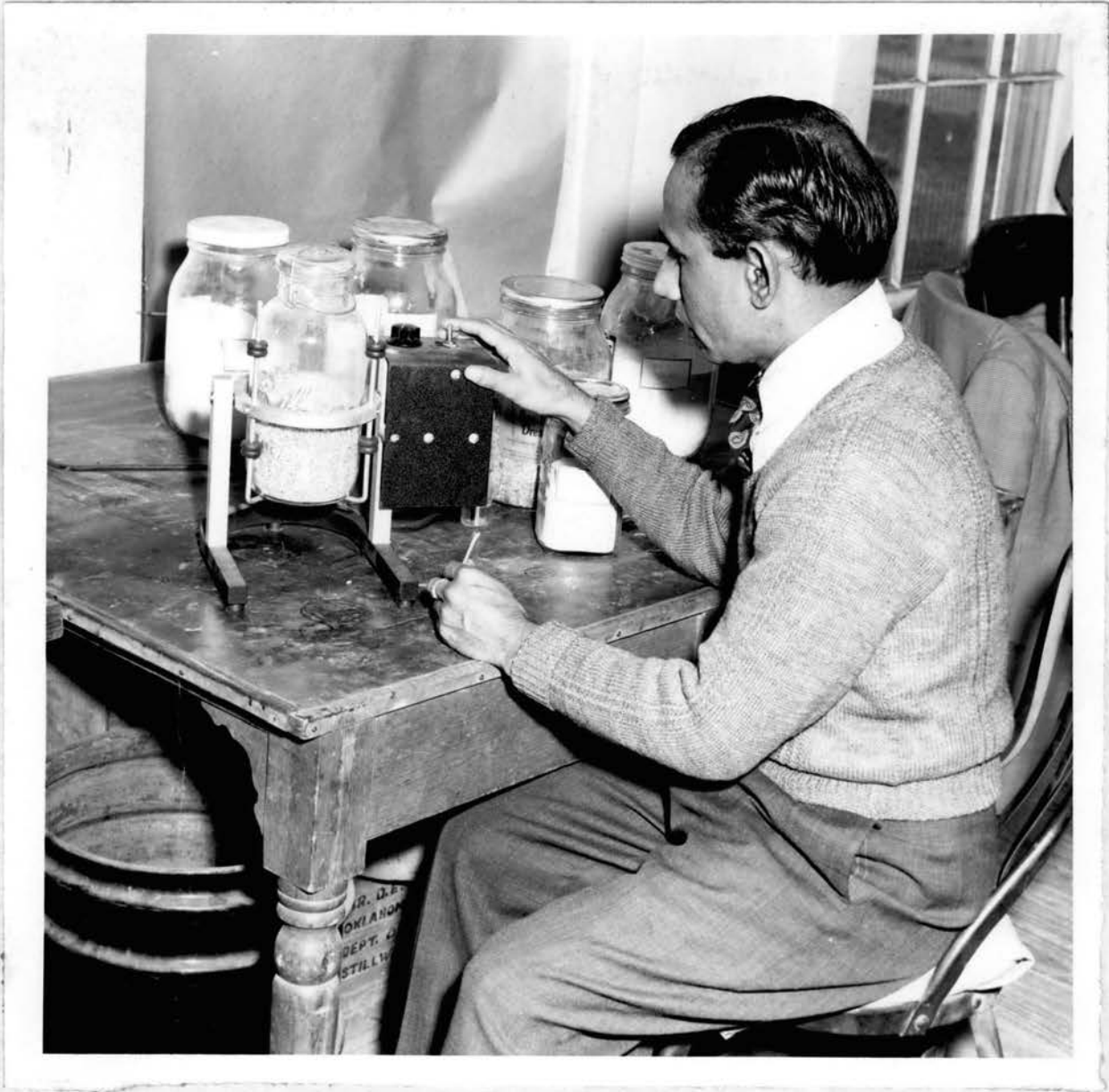
Fig. 2. Mixing an Insecticide with the Grain on the Standard Ball Mill.
