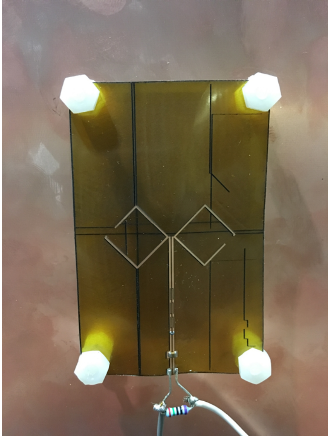
Figure 5.3: Photo of Final Rectenna with Diode, Capacitor and Resistor Soldered
