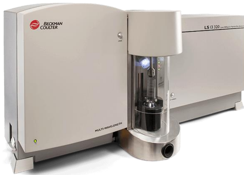
Figure 16: Dry laser particle size analyzer (Beckman Coulter 2013)
