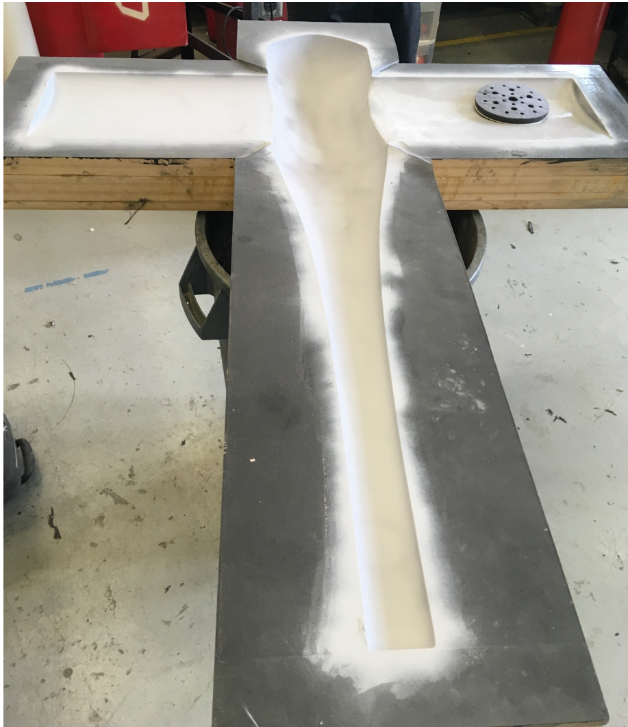
Figure 3.9: Image of Top Fuselage Mold Coated with Primer
