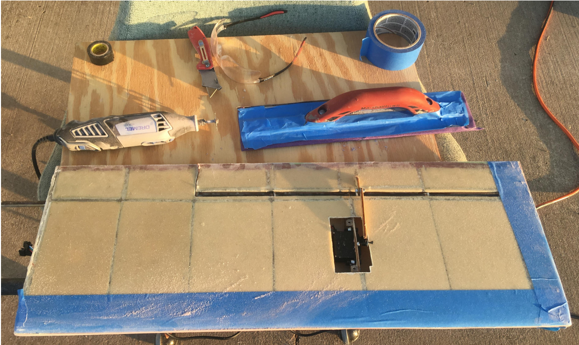
Figure 3.16: Image of Outer Wing Following Flange Trimming
