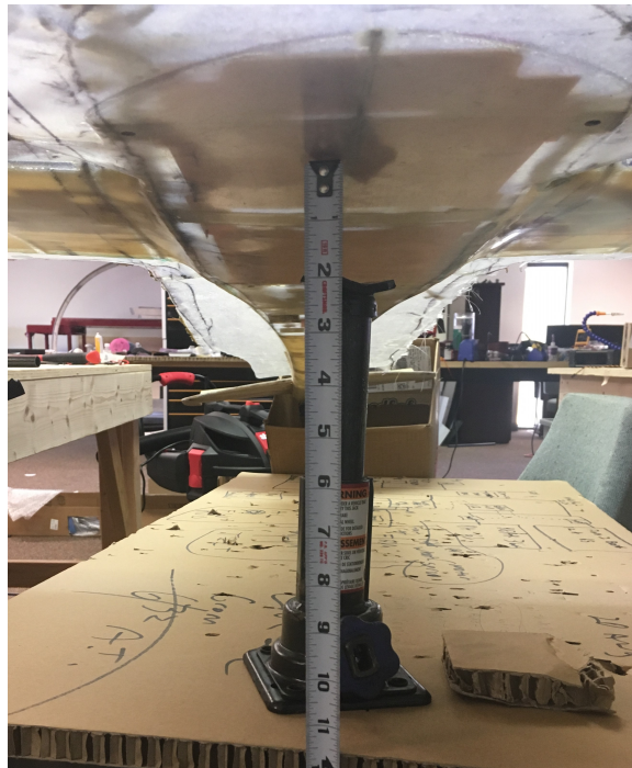
Figure 4.5: Image of Initial Tip Test Sag
