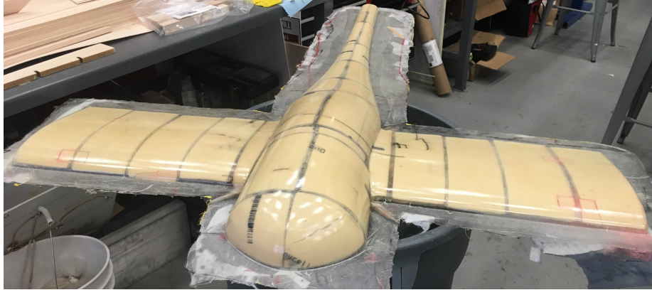
Figure 3.12: Image of Cured Top Fuselage Skin
