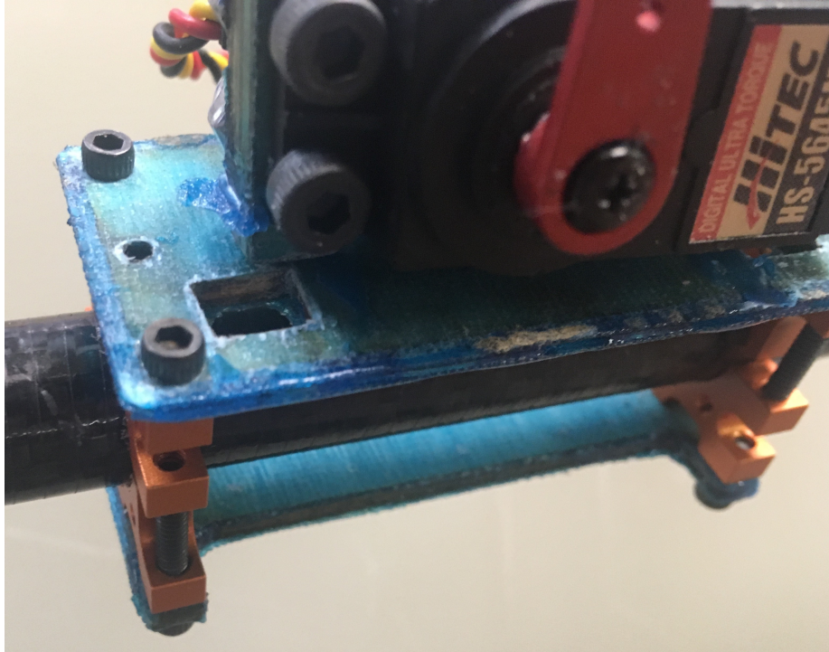
Figure 4.2: Image of Servo Platform Failure
