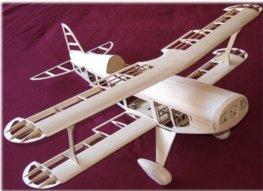
Figure 1.32: Balsa Construction of Model Pitts S2B (Carpenter 2018)
