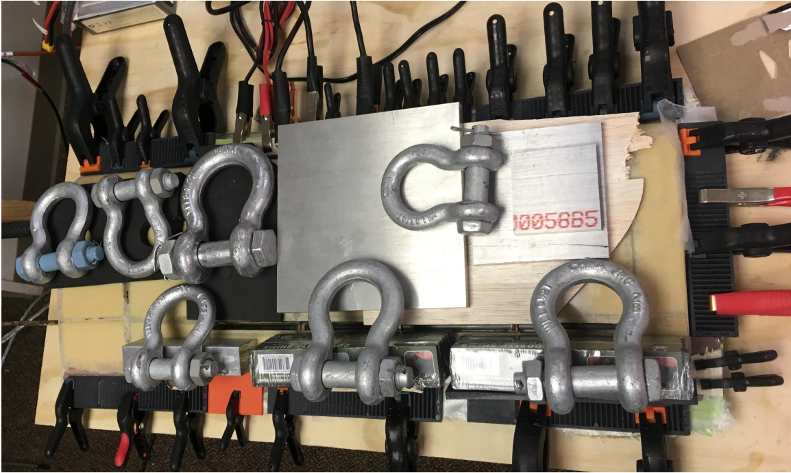
Figure 3.15: Image of Outer Wing Following Sandwiching
