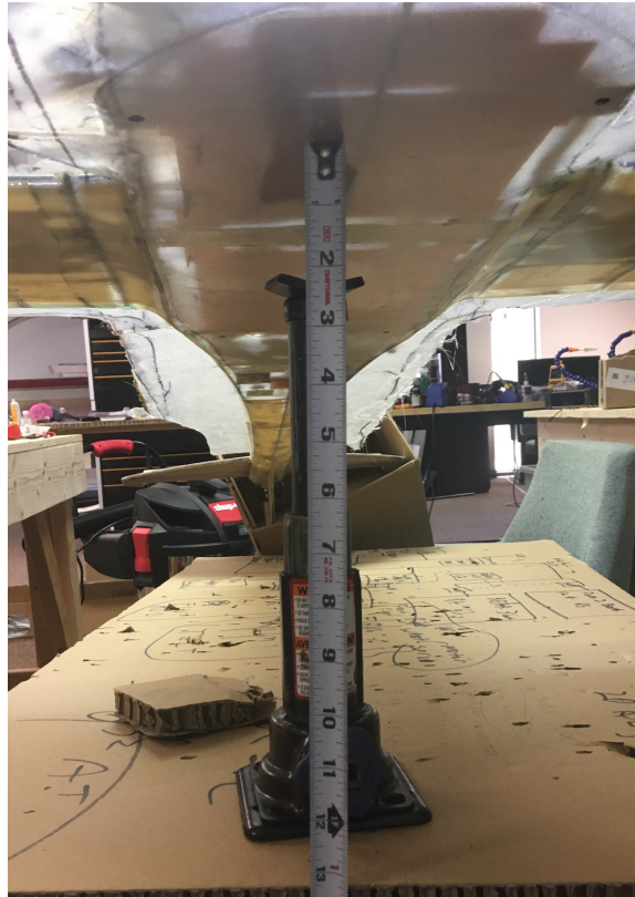
Figure 4.6: Image of Spar-Reinforced Tip Test Sag
