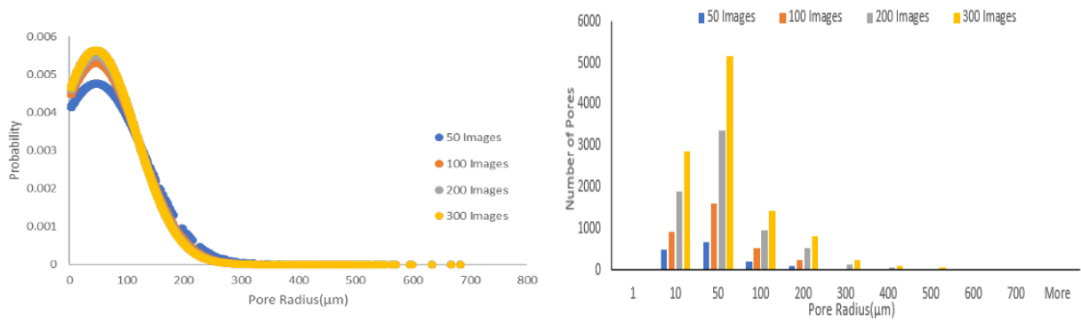
Figure 56 (a) Pore Radius Distribution Function (b) Histogram of Pore Radius for Sandstone S8 Sample
