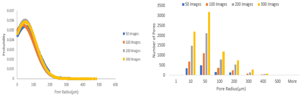
Figure 54 (a) Pore Radius Distribution Function (b) Histogram of Pore Radius for Sandstone S6 Sample
