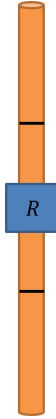
Figure 5.4: Example of wire antenna now with the addition of a time-varying load
