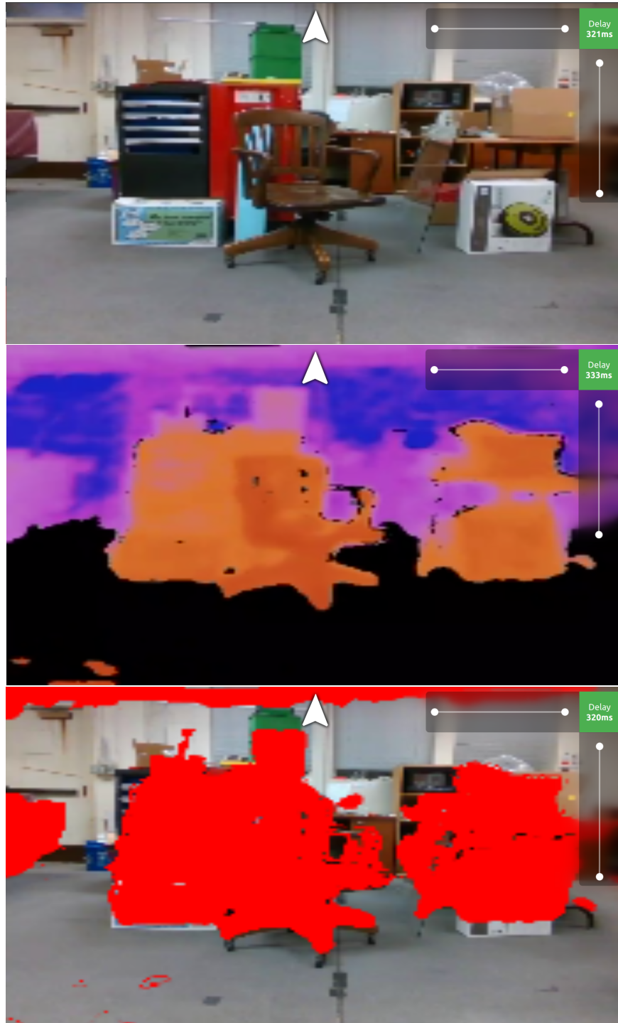
Figure 4.13: (Top) Input image to AR pipeline; (Middle) depth image of scene after ground filtering; (Bottom) final image delivered to user with AR overlay.
