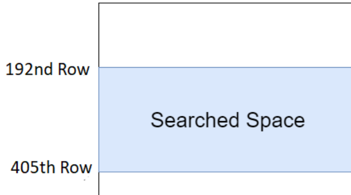
Figure 4.12: Space searched for ground by ground detection - algorithm searches from 192nd row of image to 405th, and cuts off all other rows in image.
