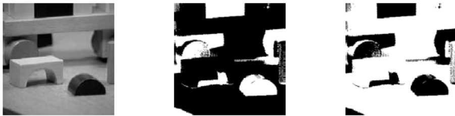
Figure 4.1: Example of a pixel thresholding filter applied to a grayscale image showing, from left to right, the original image, a threshold below operation on that image with t=93 , and a threshold above operation with the same t value. [31]
