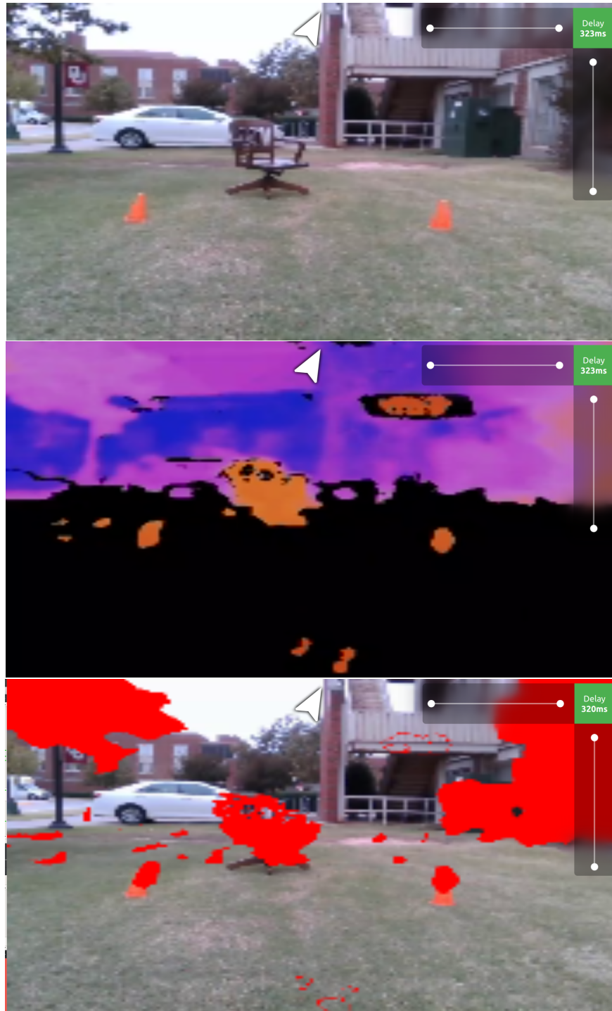
Figure 4.14: (Top) Input image to AR pipeline; (Middle) depth image of scene after ground filtering; (Bottom) final image delivered to user with AR overlay.
