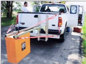
Figure 3.20: The GPR Equipment Used at Tar Creek Site
