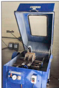
Figure 3.6: Heavy Duty Asphalt Saw
