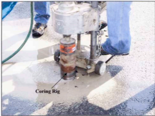
Figure 3.3: Field Asphalt Coring Machine
