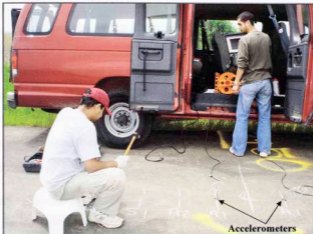
Figure 3.22: A Photographic View of a SASW Test
