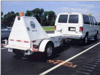
Figure 3.17: FWD Device Used in the Davis and Eastern Ave. Project Site
