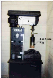
Figure 3.7: Heavy Duty Laboratory Coring Machine
