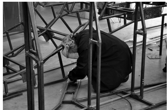
Fig. 1. Welding Frame Components. University of Houston MicroLiving Studio. Photo by S. R. Perez.
