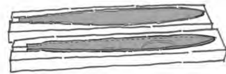
Step 2: Lay-up resin and fiber mixture on each part of the mold. Make sure there will be an overlap between the lay-up when the mold is closed.
