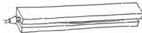
Step 4: Close mold, taking care to push the layers of fiber and resin into the mold. Clamp the mold and inflate the bladder. Keep mold closed until FRP cures.
