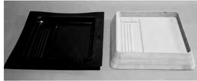
Fig. 5. On the right is an MDF pattern used to thermoform the plastic. On the left is the plastic mold that is formed and ready for casting. Photograph provided by Victor Galloway III.
