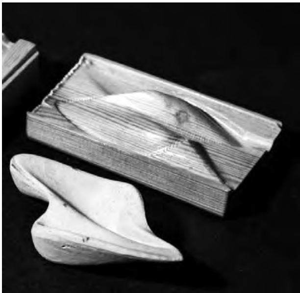
Fig. 3. A close-up photograph of the smallest iteration. Note the air bubbles on the sides of the unit due to the orientation of the pour. Photographs provided by Hengchen Liu.
