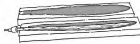
Step 3: Place bladder inside of mold.
