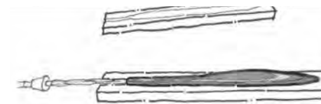
Step 5: Open mold, deflate, and remove bladder.
