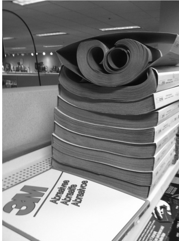
Figure 26 – Curl Due to Humidity
