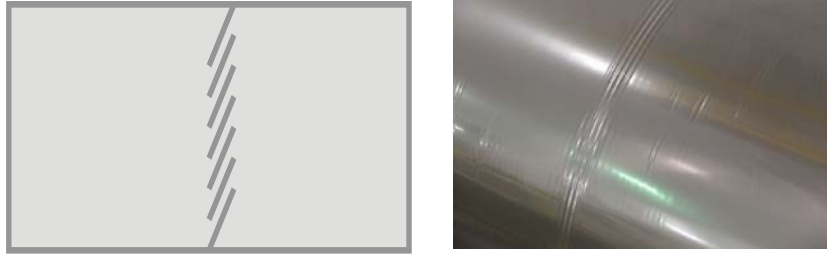
Figure 2 – Corrugation Caused by a High-Low-Medium Caliper
