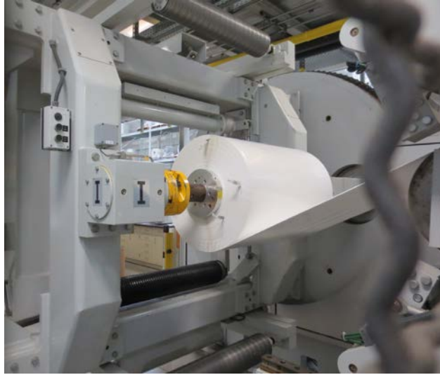
Figure 5 – Machine Set Up for Laminate Web Winding Tests
