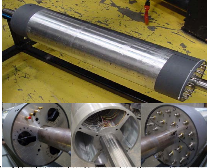
Figure 13 – A Core Instrument for Measuring Core Pressure. Top: Assembled Core, Bottom Left: Switchable Output, Bottom Center: Instrumented Rings and Bottom Right: Bridge Balance.
