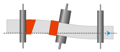
Figure 2 – Stresses on the outside of the bend due to inplane roller misalignment
