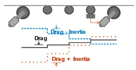
Figure 1 – Downweb stress profile due to bearing drag and inertia
