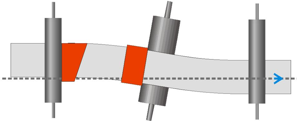
Figure 2 – Stresses on the outside of the bend due to inplane roller misalignment
