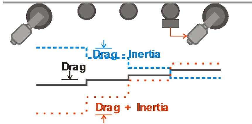
Figure 1 – Downweb stress profile due to bearing drag and inertia
