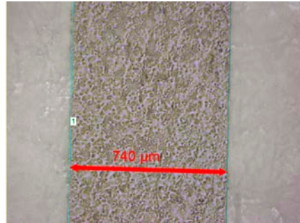
Figure 18 – Measurement lines under microscope on bars (printed element)
