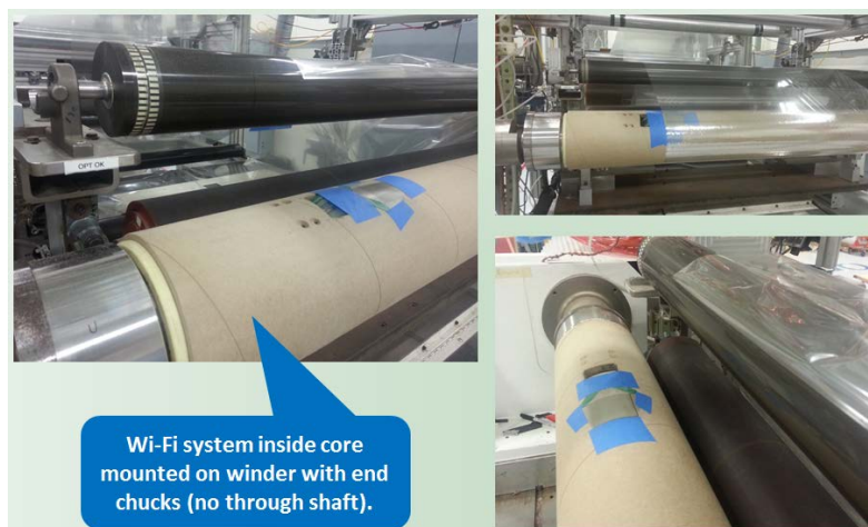
Figure 4 – Equipment on Winder Mounted Inside of Core
