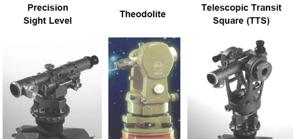
Figure 1 – Foundations of alignment tooling - Courtesy OASIS
