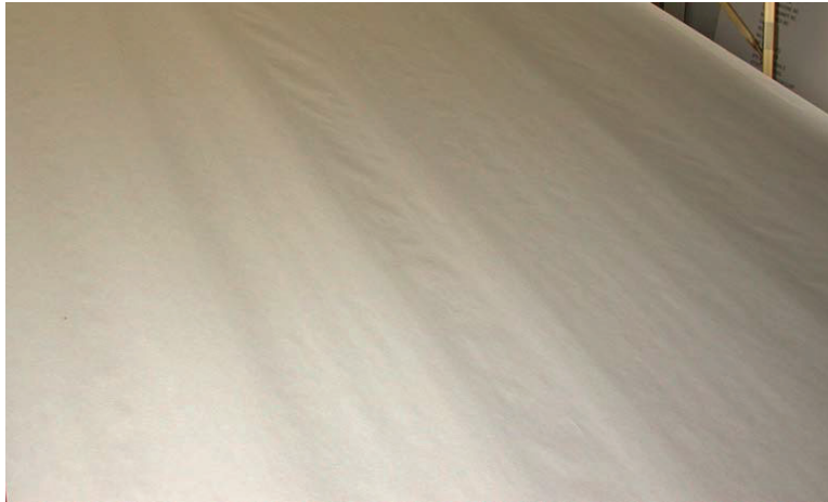
Figure 15 – Narrow baggy streaks issue across the width of super-calendered paper
