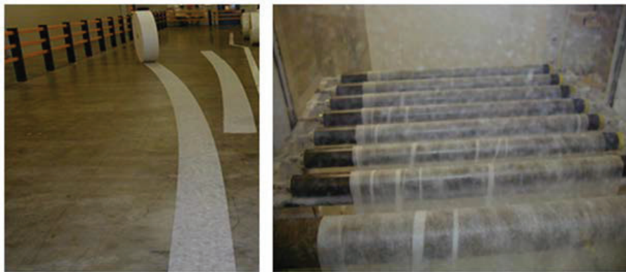
Figure 1 – Cambered web and wrinkles in an accumulator
