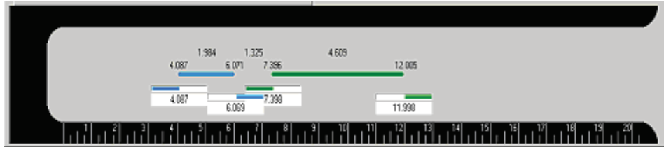
Figure 24 – Two webs with overlapping 2 inch virtual sensors (edge polarity)
