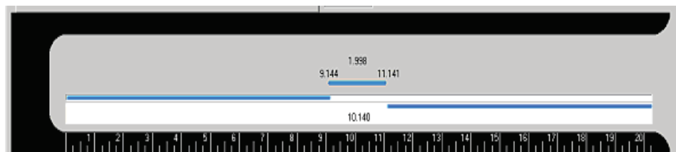
Figure 22 – Center-guiding a single web with two overlapping 20.28 inch virtual sensors
