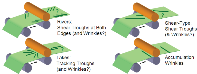
Figure 6 – Buckled Web in Spans near Nips
