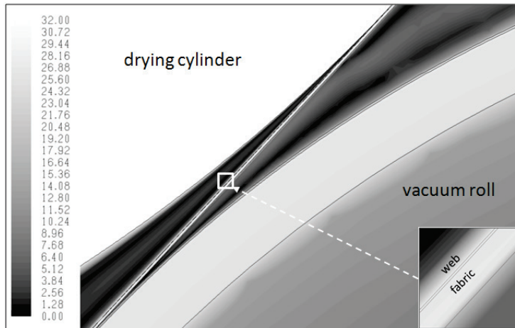
Figure 7 – Steady-state velocity profile (m/s) and initial web/fabric position
