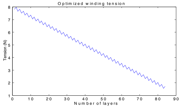
Figure 8a - Linear reference tension with dispersion ( c=\pm 1 )
