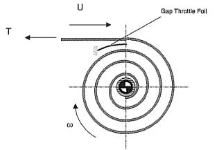
Figure 1 Sketch of a gap throttle foil in the winding process
