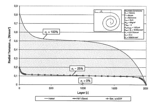
Figure 6 – Radial tension calculated with the model of Hakiel, Good and the new gap throttle model
