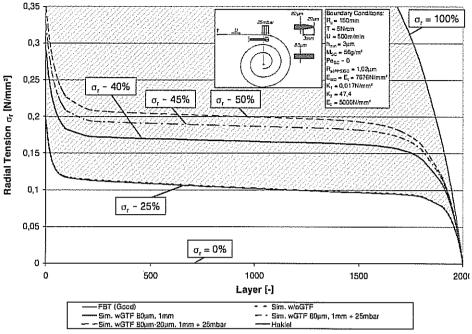
Figure 9- Radial tension without and with gap throttle foil resp. with support pressure
