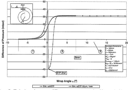
Figure 7 - Hydrodynamic pressure difference versus wrap angle without and with gap throttle foil
