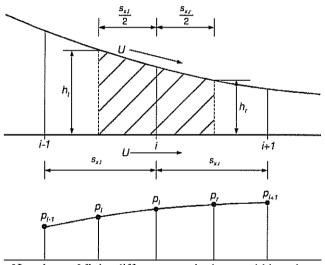
Figure 4 - Notations of finite difference method, gap width and pressure [13]
