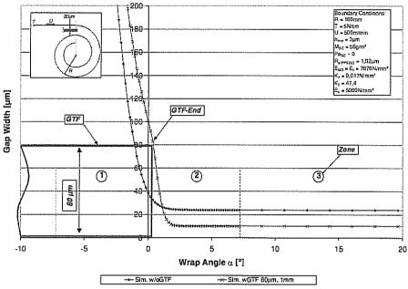
Figure 8 - Gap width without and with gap throttle foil
