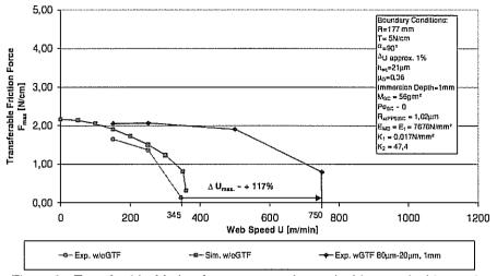
Figure 2 - Transferable friction force versus web speed without and with gap throttle foil(GTF)
