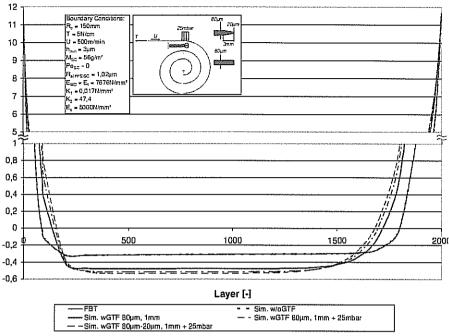
Figure 10 - Tangential tension without air entrainment, without and with gap throttle foil and with support pressure
