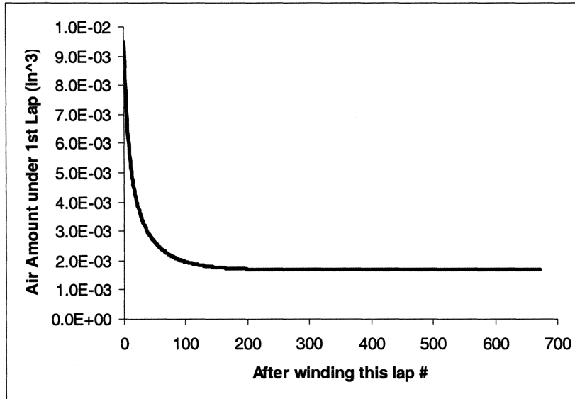
Figure 8 – The amount of air (adjusted to ambient air pressure) left under 1 st lap during winding.
