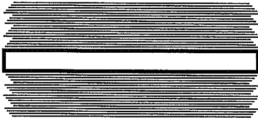
Figure 9 - Sawtooth Edges Due to Nip Friction
