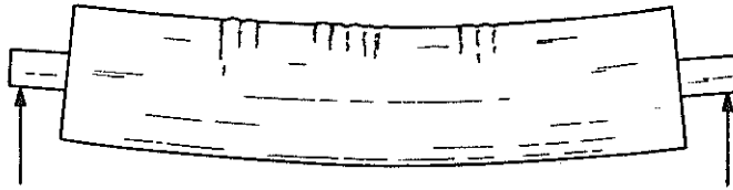
Fig. 8 Corrugations at top of simply supported roll
